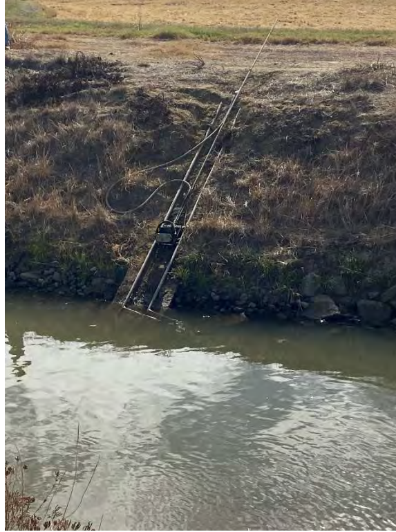
Figure 14. Existing GCID Sontek SL out of the water.
