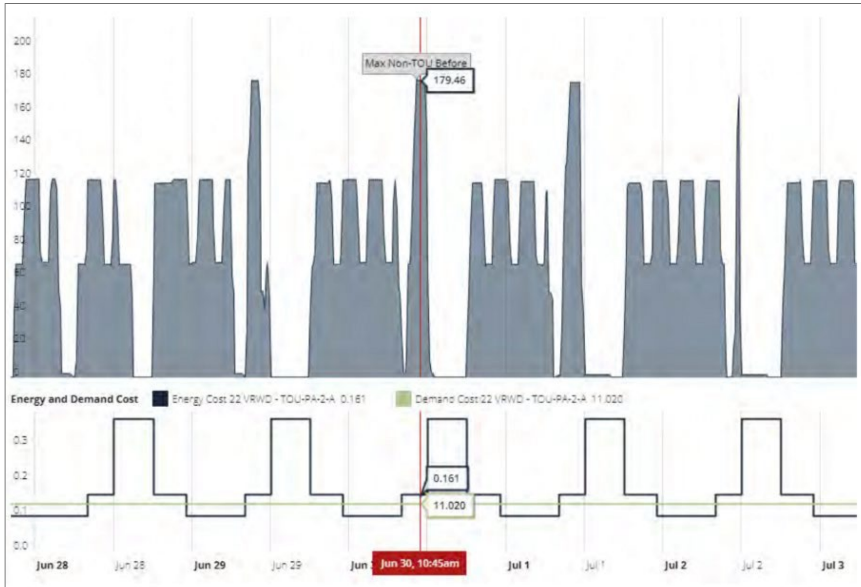
Figure 8: Baldwin Pump Station Energy Usage Profile, Battery Effect Removed
