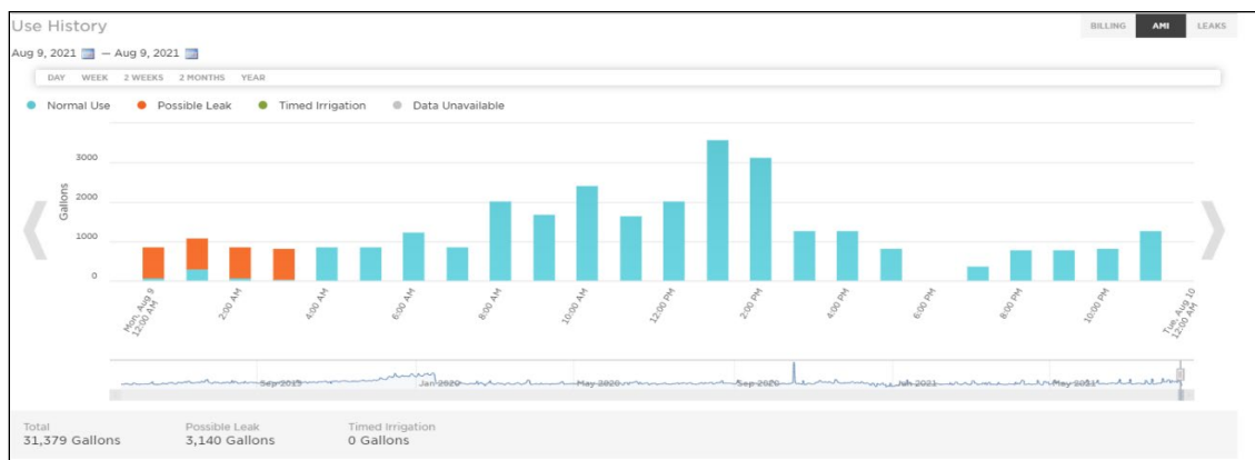
Figure 11. Hourly data showing continuous water consumption which is likely a leak
