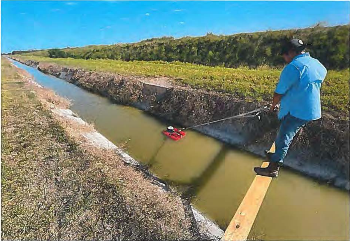
Figure 3.2: Measuring of Water Current Velocities at the North Crossover Main Canal
