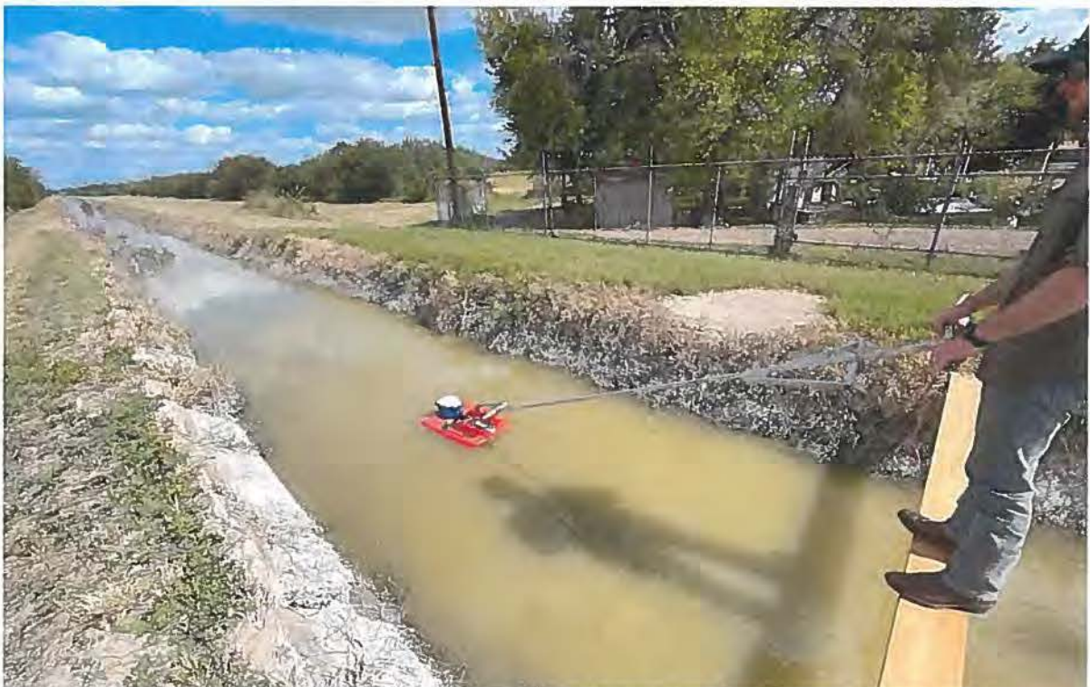
Figure 3.1: Measuring of Water Current Velocities at the East Main Canal
