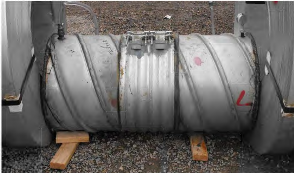
Figure 15: Photo of Contech testing of Ultra Flo pipe with 5C bands
