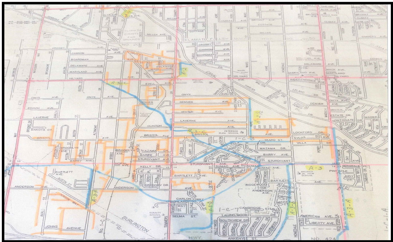
Figure 19 Suburban Private Ditches (in orange) which need NRCS efficiency improvements within Klamath ID
