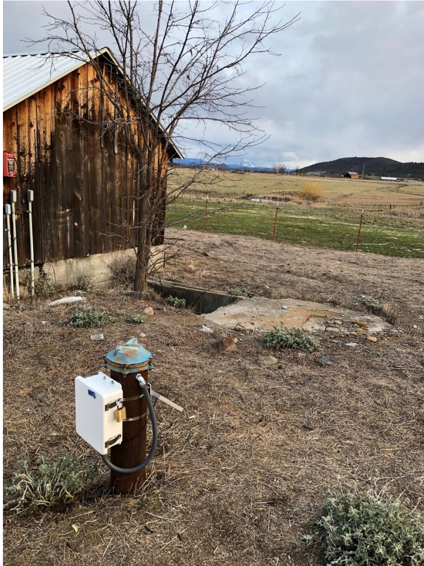
Figure 2 Installed groundwater data logging equipment with telemetry and compact solar array
