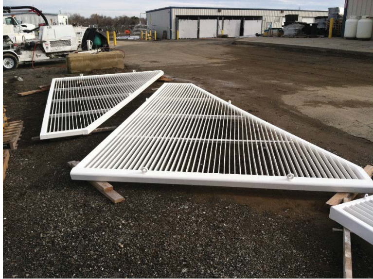
Figure 2. Trash Rack for canal siphon, post fabrication.
