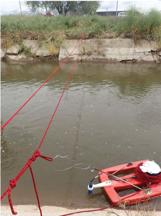
Figure 8 – Mid-stream measurement location data collection setup. Note highly fractured concrete liner. ADCP is mounted in boom position.
