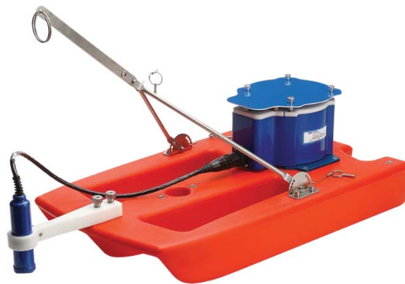
Figure 4 – Teledyne RD Instruments' StreamPro ADCP. Similarly equipped to model used. [Teledyne Marine, 2004].
