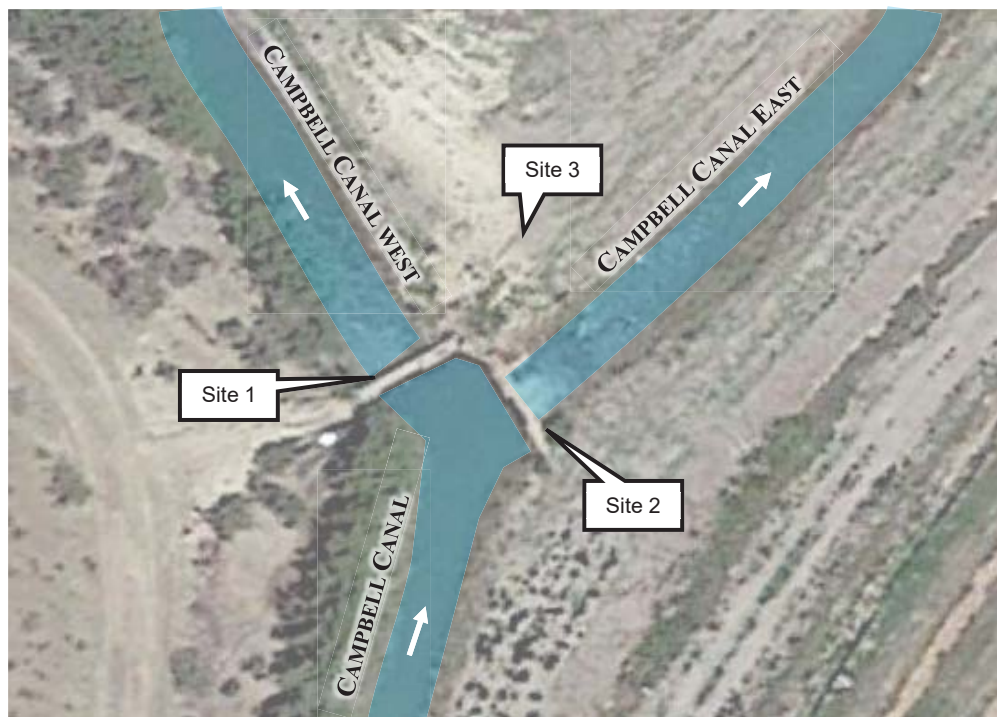
Figure 6. Layout of the proposed upgrades to the Campbell Canal Split
