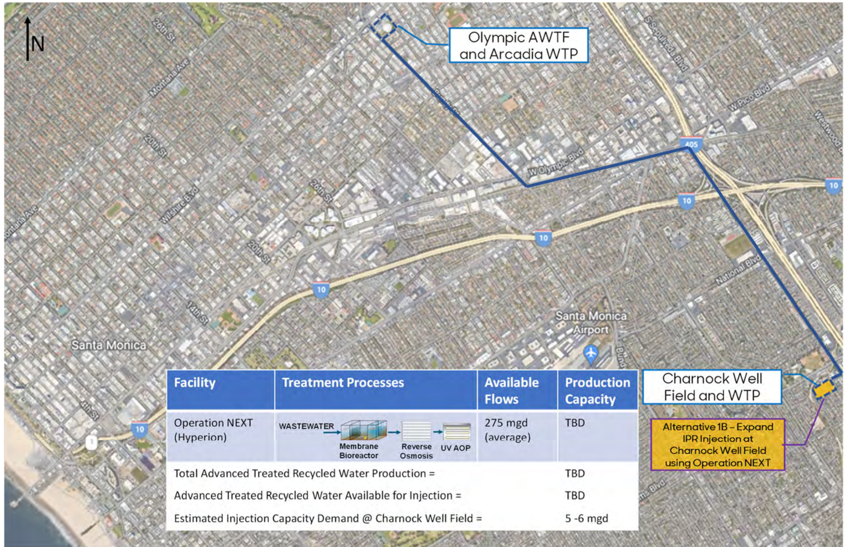
Figure 3: Summary of Alternative 1B – Expand IPR at Charnock Well Field with Operation NEXT
