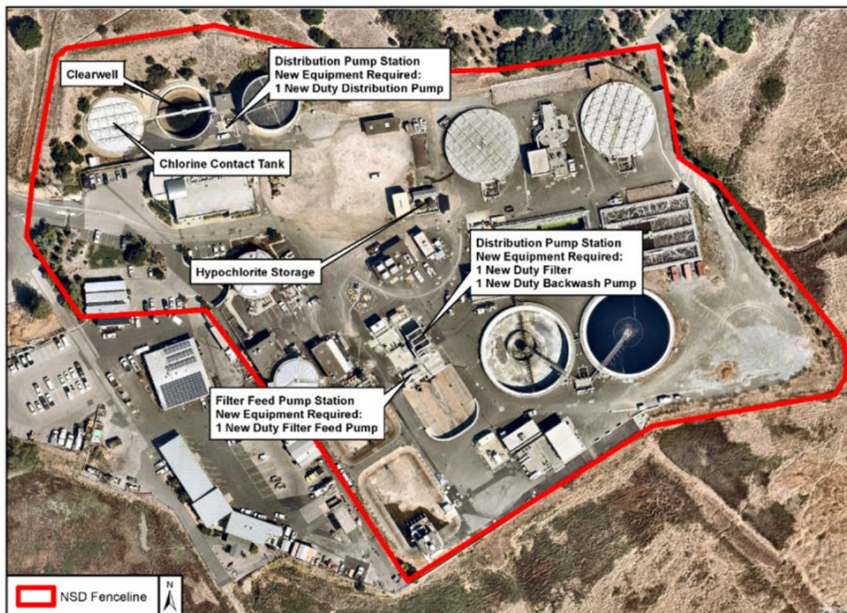
Figure 3. North Central Service Area Treatment Facilities – Existing NSD RWF Process Structures with New Equipment Required to Increase Capacity to 1.7 mgd
