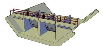
*Figure 2. 3D rendition of a two bay radial gate check structure*
