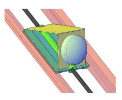
Figure 6. 3D representation of a sliding mount for an acoustic doppler sensor.
