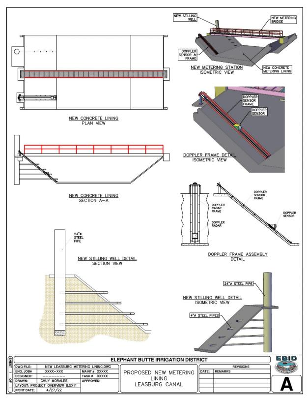
Figure 4. Design components of proposed Leasburg Canal metering site
