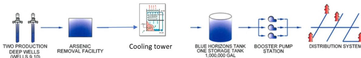
**Figure 3-1 Schematic of Blue Horizons Treatment Facility**
