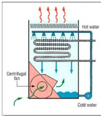
**Figure 3-1 Closed Loop Cooling Tower Schematic**
