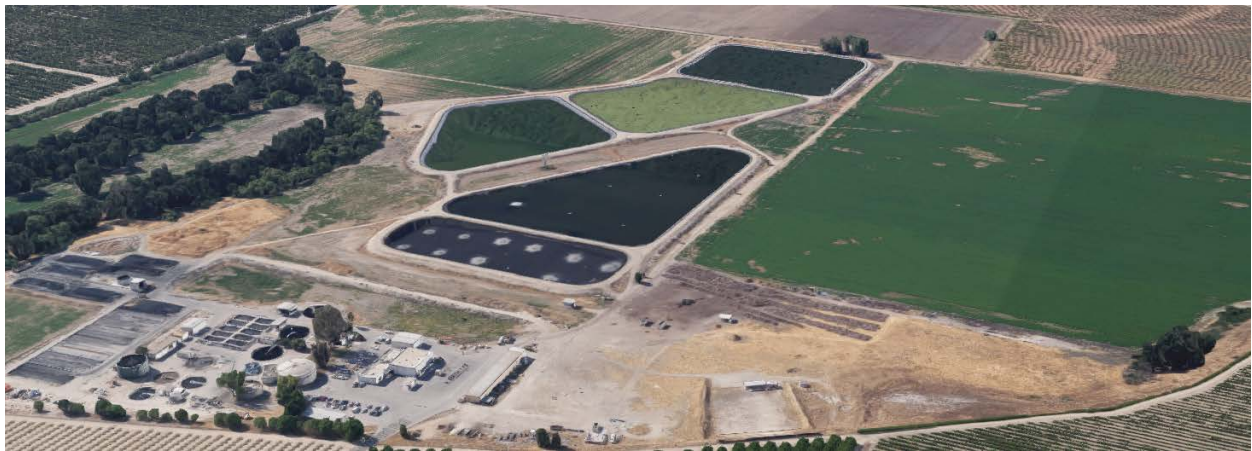
Treated wastewater, in percolation ponds and applied to crops, helps to recharge the groundwater basin at the Sanger wastewater treatment plant.
