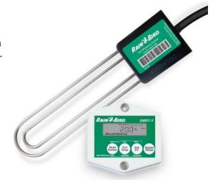
sufficiently high, the SMRT-Y will disable all zones from irrigating. The SMRT-Y acts as a switch, opening and closing the zone common wire depending on the soil moisture level. When the zone common wire is open, the irrigation system valves will not operate. The moisture threshold—the level of moisture where the SMRT-Y switches on or off—is set by the user and can be adjusted up or down as needed.
