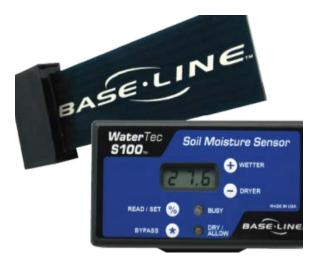
appropriate for outdoor installation. Its dimensions are 4.6 by 2.6 by 1.5 inches, and it has a three-character, one-line LCD and touchpad-type controls. The WaterTec S100 comes with a 6-inch biSensor soil moisture sensor.
