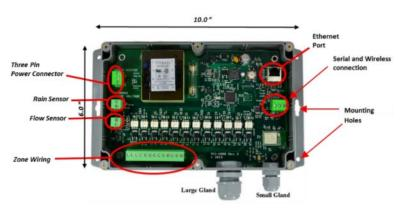
a/b/g/n or a hardwired, Ethernet connection. The unit can connect to a master valve or booster pump. Physically, the unit measures 10 inches long by 6 inches high by 3.5 inches wide. The unit is intended to be wall-mounted.
