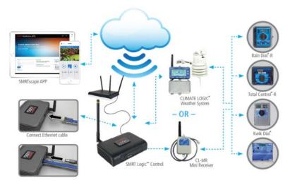
gateway. The service is managed and accessed through the  $Toro^{\$}$ -Irritrol $^{\$}$  website (SMRTscape.com). The SMRT  $Logic^{TM}$  Hub can also be connected to compatible wireless lighting controllers.
