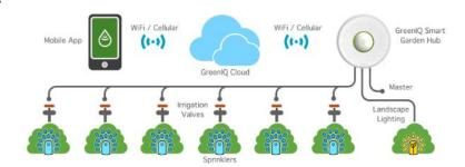
circuit. The Smart Garden Hub is designed for indoor installation, but an outdoor IP55 waterproof box is approved for outdoor use. The dimensions for both models are 6.3 inches in diameter and 1.06 inches in depth.
