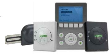
landscapes. The UgMO Solution uses UgMO wireless soil sensors to ensure that only the amount of water needed by a landscape is applied.
