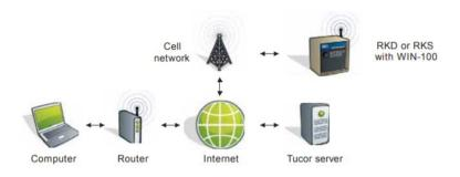
use with the end-user's LAN), which can be hardwired or be a part of a 900-MHz radio network. RealNet also allows for interaction with a controller via Tucor's companion smartphone and tablet Java-based app. Through this app, the user can, among many things: start and stop programs and stations, verify real-time flows, and check the controller's electrical status.
