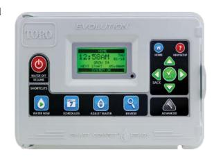
smartcontroller (weather-based scheduling), the EVOLUTION® controller must be paired with the Wireless ET Weather Sensor (model EVO-WS), the EVOLUTION's® onsite weather station. The Wireless ET Weather Sensor collects temperature, rain, and solar-radiation data that are transmitted directly to the EVOLUTION® controller via a Smart Connect® receiver.
