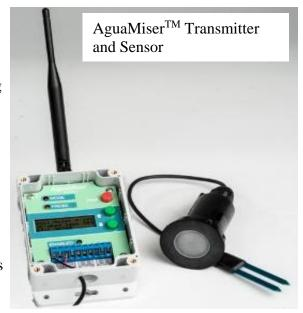
bound. AguaMiser technology interprets sensor readings and adjusts the state of the relays that will accommodate "N/O" (normally open) or "N/C" (normally closed) circuits. This allows the user to adapt to a multitude of situations; such as, using this technology to start fertigation systems or even control SCADA and other protocol-type switches.
