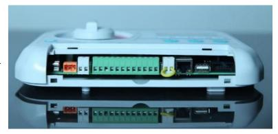
station 12 dedicated as a master valve or pump start. Model HWN12-200 provides a rain sensor and 10-pin port, which connects to the 24-zone extension module (model HWN24-2EXT).
