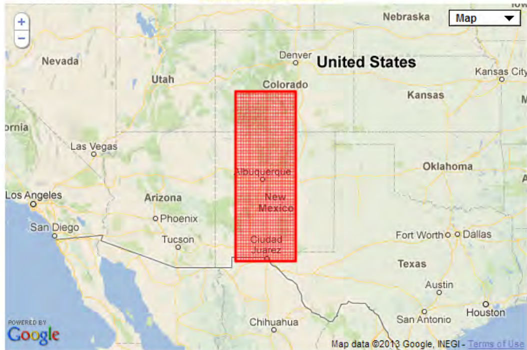
Figure 1: Spatial area used to define the average temperature and precipitation value for each GCM for a given time period. Extents are 31.6875 through 38.5625 degrees of latitude, and -107.9375 through -105.0625 degrees of longitude. Screen capture is from http://gdo-dcp.ucllnl.org .
