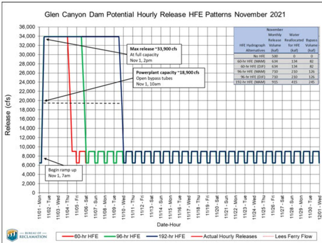
**Figure 3. November 2021 Schedule of Releases for Alternative Fall HFE Hydrographs**
