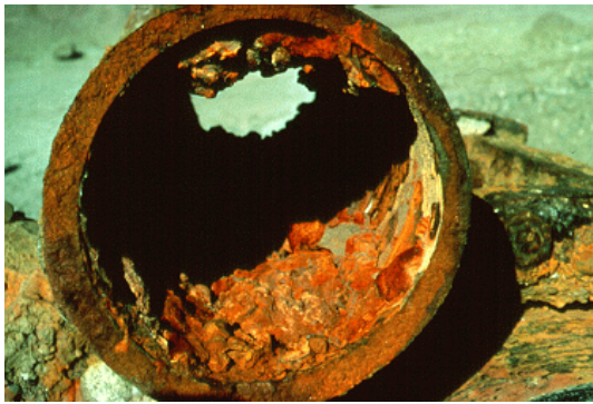
Salinity damages to municipal water pipe.
