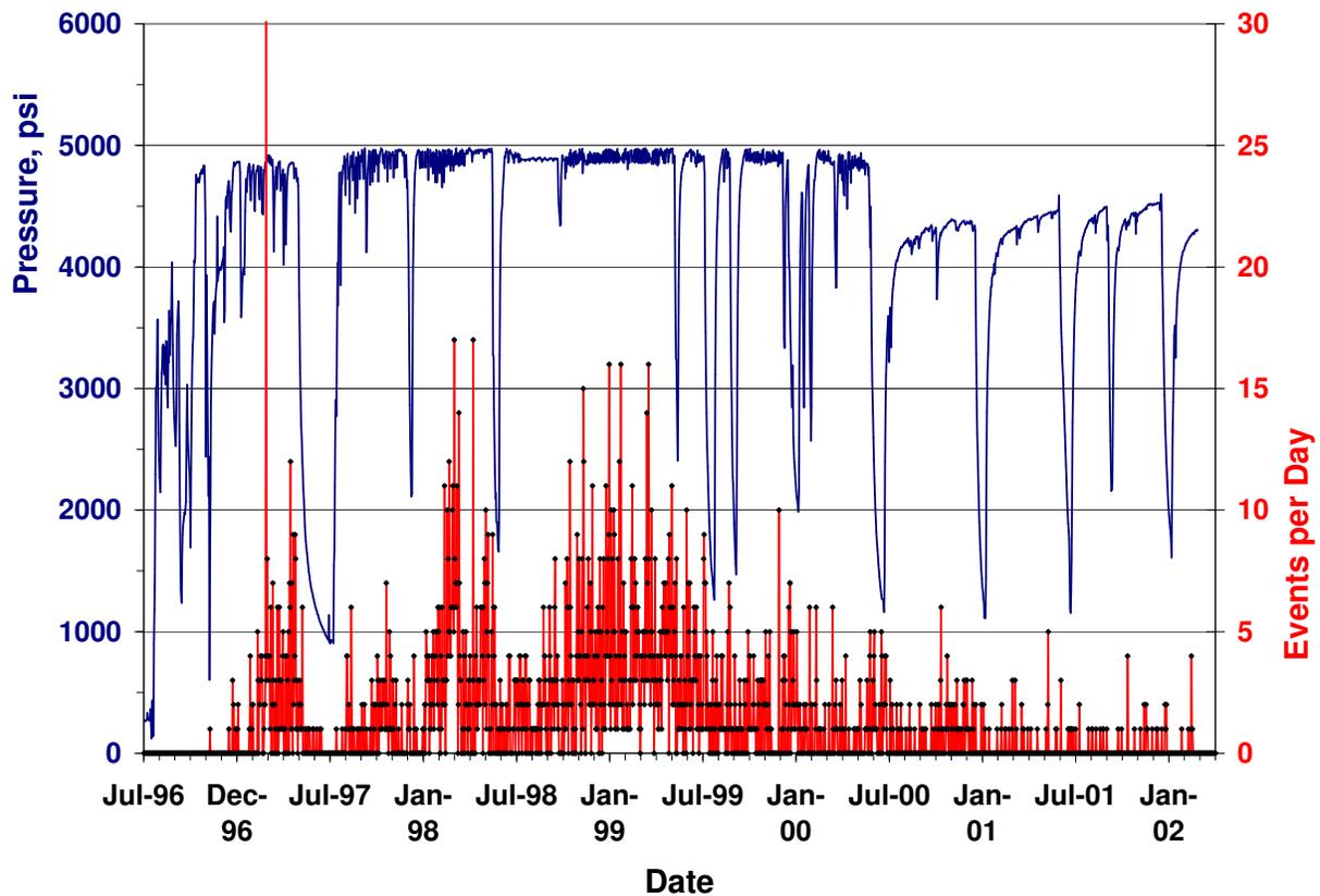
*Figure 7. Number of events per day (red) and surface injection pressure (blue) versus time.*
