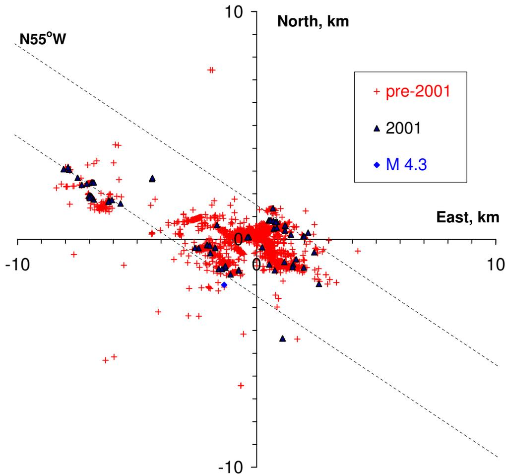
*Figure 10. PVU-induced earthquake epicenters for 2001 and years 1998-2000. All epicenters are relocated from one-dimensional model. Axes are centered on the PVU injection well. Dash lines run N55°W, the implied strike of Wray Mesa Fault system.*
