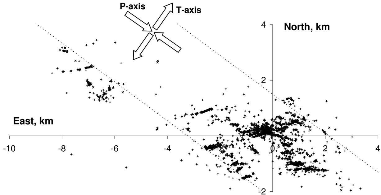
*Figure 17. Close up of relocated seismic epicenters. Axis is center on injection well. Dashed lines run N55°W, the assumed strike of the Wray Mesa Fault system. Linear groupings of epicenters show (implied) seismically-activated faults and (pre-existing) fractures.*
