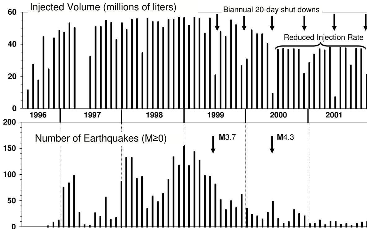
*Figure 5. Monthly injection volume (top) and monthly earthquake production at PVU versus time. Noted are onsets of bi-annual, 20-day shut downs, reduced injection rates and the M3.7 and M4.3 earthquakes.*
