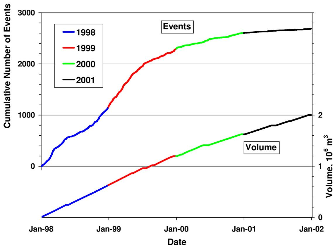
*Figure 4. Cumulative number of seismic events and cumulative injection volume versus time. Flat portions in volume curve are shutdown periods (i.e., no injection). Note correspondence between many of the shutdowns and the change in slope (i.e., rate) of event production.*
