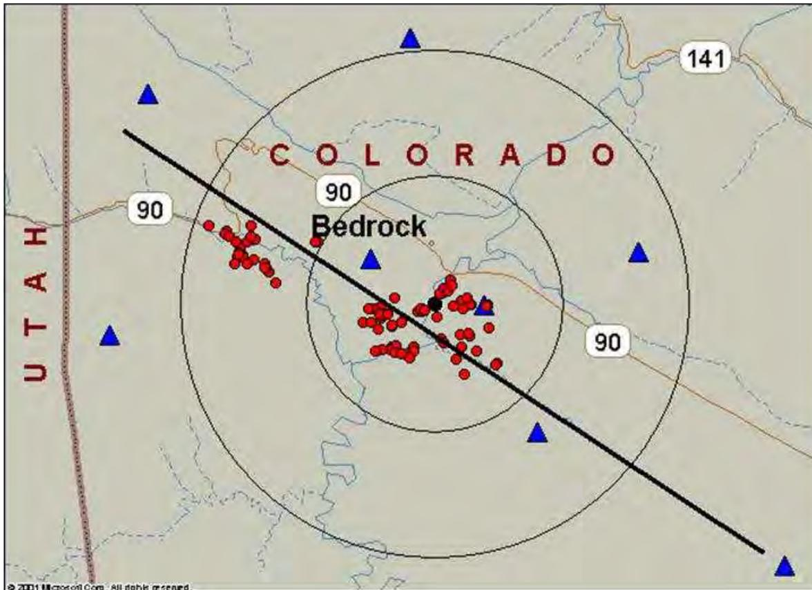
*Figure 9. Seismicity located during 2001 by PVSN using one-dimensional velocity model; 83 events plotted. Injection well is solid (black) circle. Approximate strike of Wray Mesa fault system (Bremkamp and Harr, 1988) shown as solid line. Some PVSN seismogram sites shown in filled (blue) triangles. Concentric circles are 5-km and 10km radii centered on injection well.*
