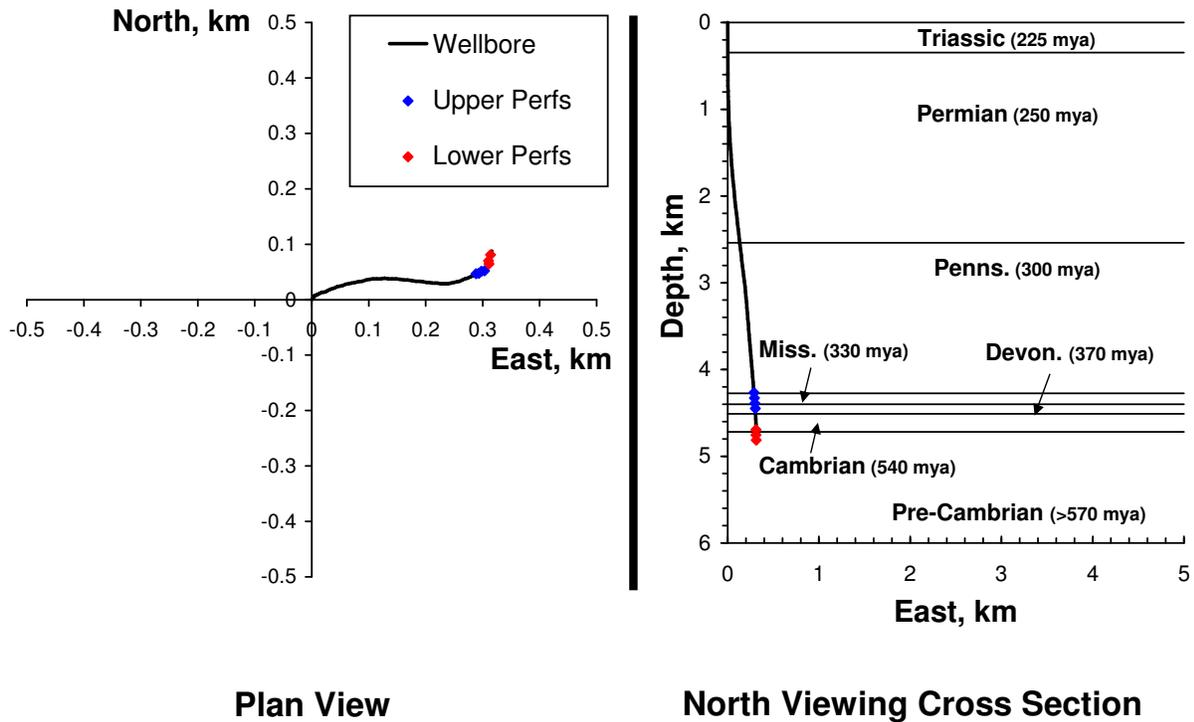
**Figure 3. Plan view and north-viewing cross section of PVU Salinity Control Well No. 1, including the stratigraphic column.**
