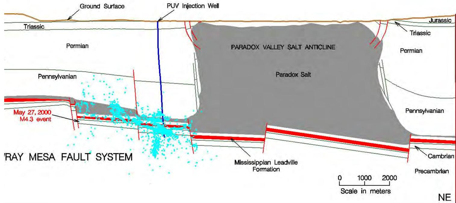
*Figure 11. Cross section of Paradox Valley and bordering region through PVU injection well and normal to strike of the valley. Projected on to cross section are all seismic events 1991 through 2001.*
