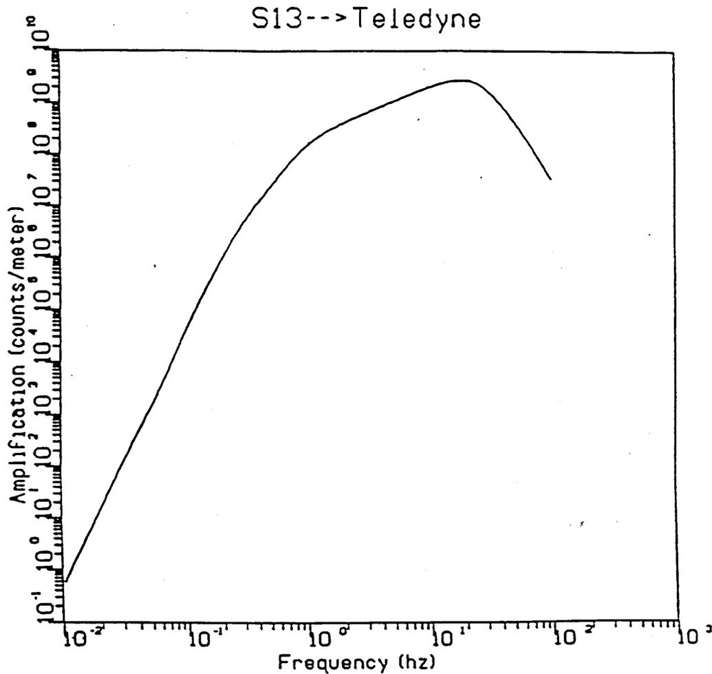
*Figure 2. Typical response of a vertical-component Teledyne Geotech S13 seismometer, electronics, and digital recording system used by PVSN. Nominal gain is 48 dB for curve shown, Teledyne Geotech model 42.5 amplifier/VCO and model 4612 discriminator. Damping is 0.71 of critical.*
