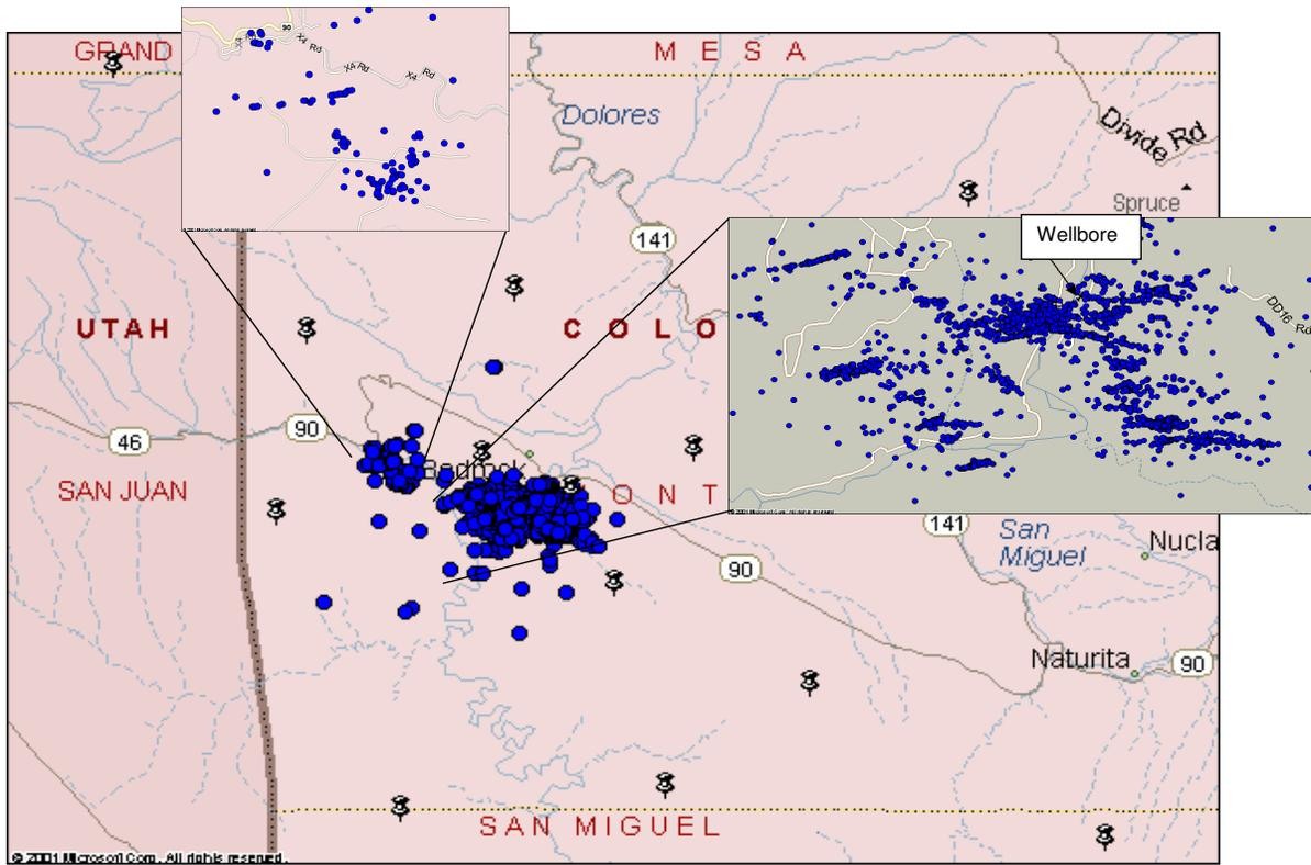
**Figure 16. Relocated seismic event locations from 1991 through 2001. Insert shows relative location of PVU injection well.**
