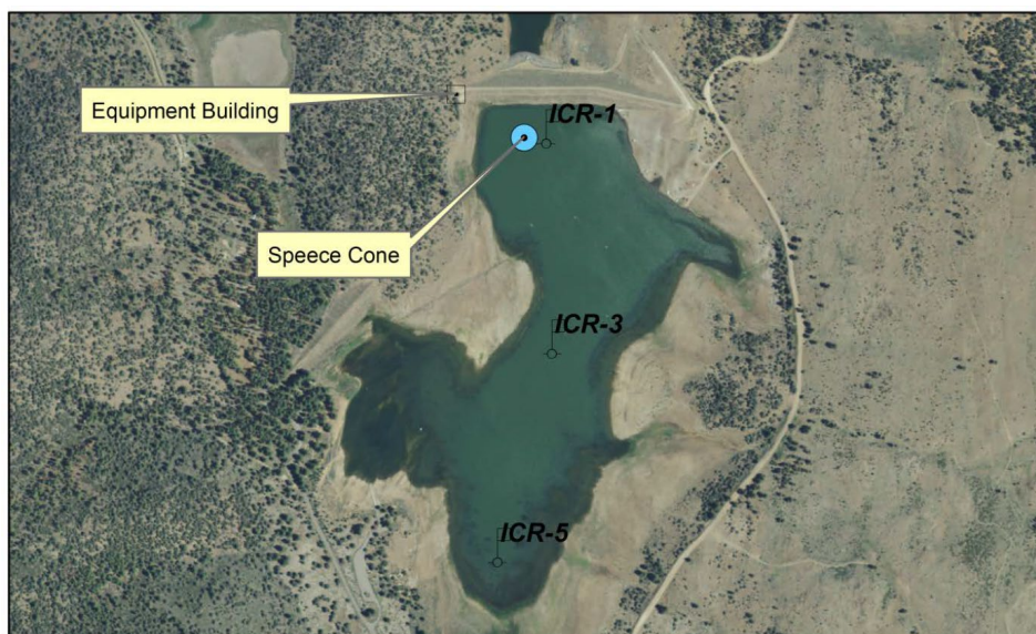
Figure 3.—Location of monitoring stations (ICR-1, ICR-2, and ICR-5), Speece cone, and equipment building where the air blowers are housed at Indian Creek Reservoir (Bergsohn 2015).
