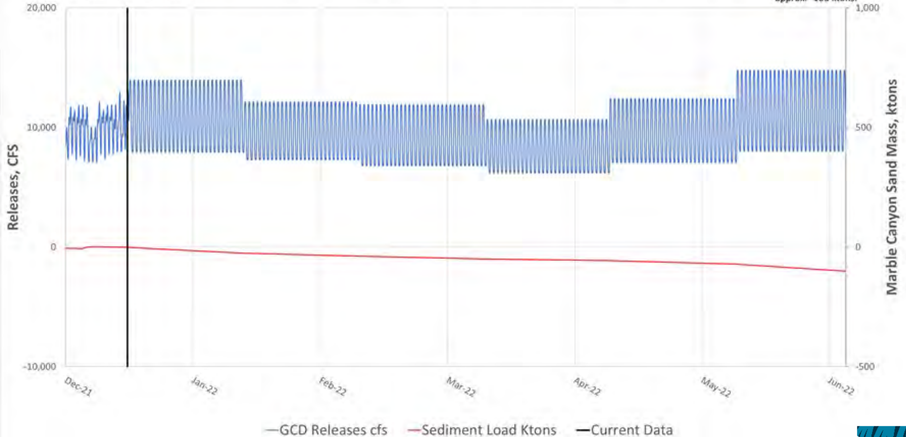
Sand Budget Model Results, Dec 1, 2021 - June 30, 2022 Release and Calculated Sediment Load in Colorado River, Marble Canyon
