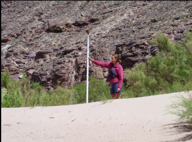
Total station surveys of exposed sand
