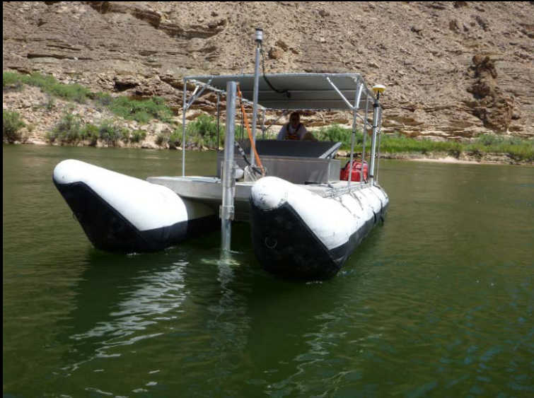
Channel bed mapping with multibeam sonar
