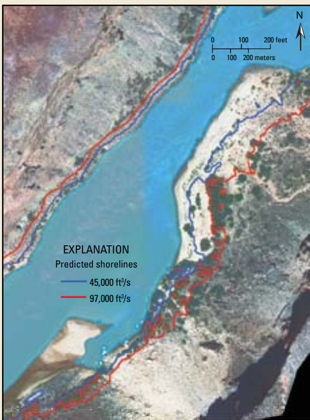
Virtual shorelines at Eminence Break camp (river mile 44). The blue shaded area (the river) shows the observed shoreline at a flow of 8,000 cubic feet per second (ft 3 /s) in the Colorado River at Lees Ferry, the blue line shows the predicted shoreline at 45,000 ft 3 /s, and the red line shows the predicted shoreline at 97,000 ft 3 /s. Modified from Magirl and others (2008).
