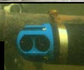
Acoustic Doppler profiler mounted in water for 15-min. measurements of sediment concentration
