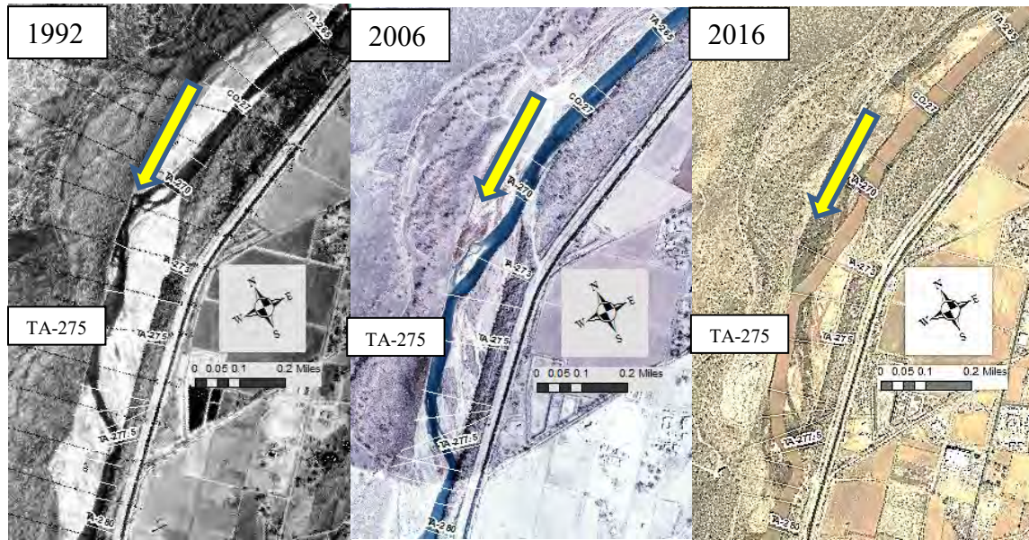
Figure 13 Near TA-275. Bend migrating downstream, resulting in a tighter meander, as the river's left bend at TA-277.5 is fixed, this location coincides with Santa Ana Projects. Yellow arrow is approximately at the same position in all images. (2)
