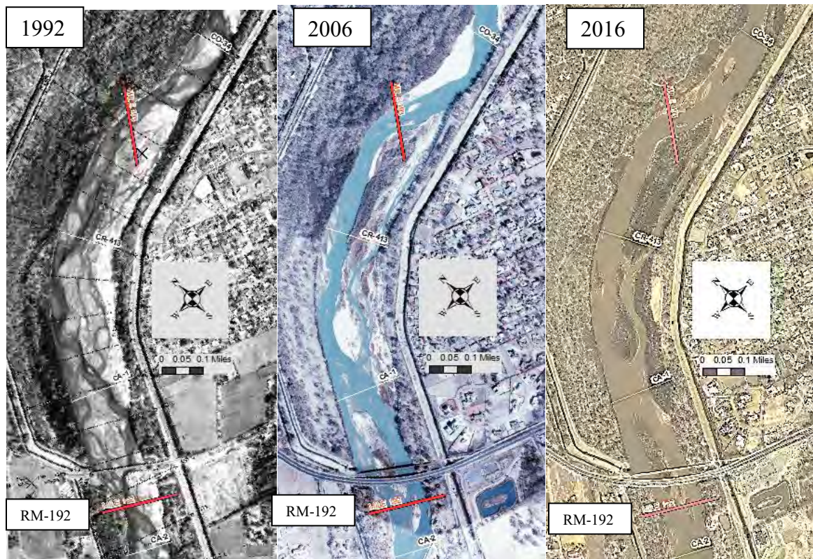
Figure 16 Changes in the planform above Alameda Bridge, where the braided planform has become established by vegetation, and connected side channels in 2016 imagery. (8).
