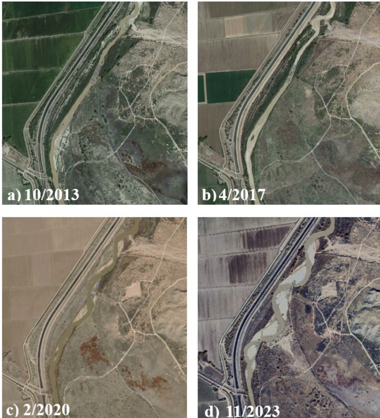
Figure 14: Satellite imagery 2013 to 2023 of bankline erosion near the Cañas Arroyo confluence.
