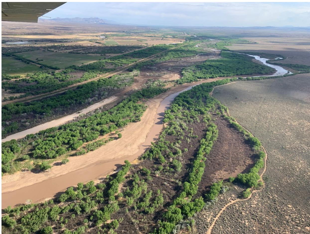
Figure 16. Image of the downstream phase of the river realignment taken in Spring 2021. Photo is looking upstream with the realigned channel to the right of the frame and the abandoned channel to the left.
