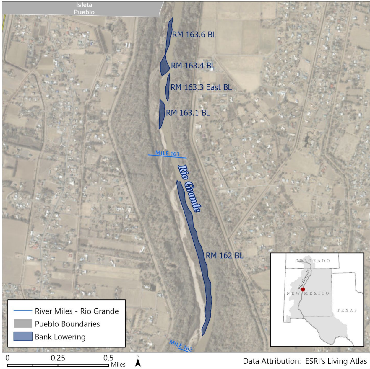
Figure 12: Plan view of bank lowering (BL) berm design for RM 163 maintenance project.
