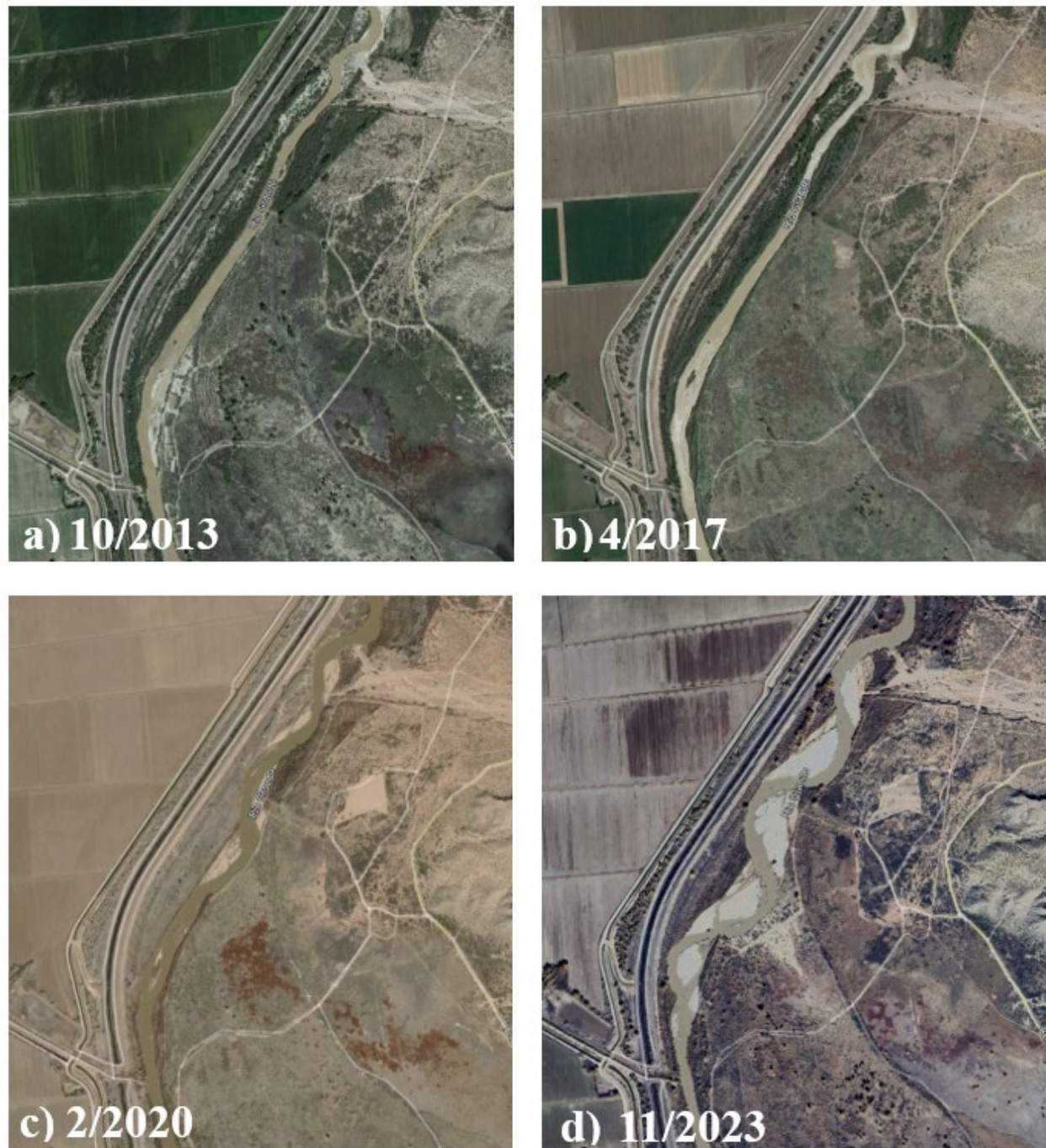
Figure 11: Satellite imagery 2013 to 2023 of bankline erosion near the Cañas Arroyo confluence.
