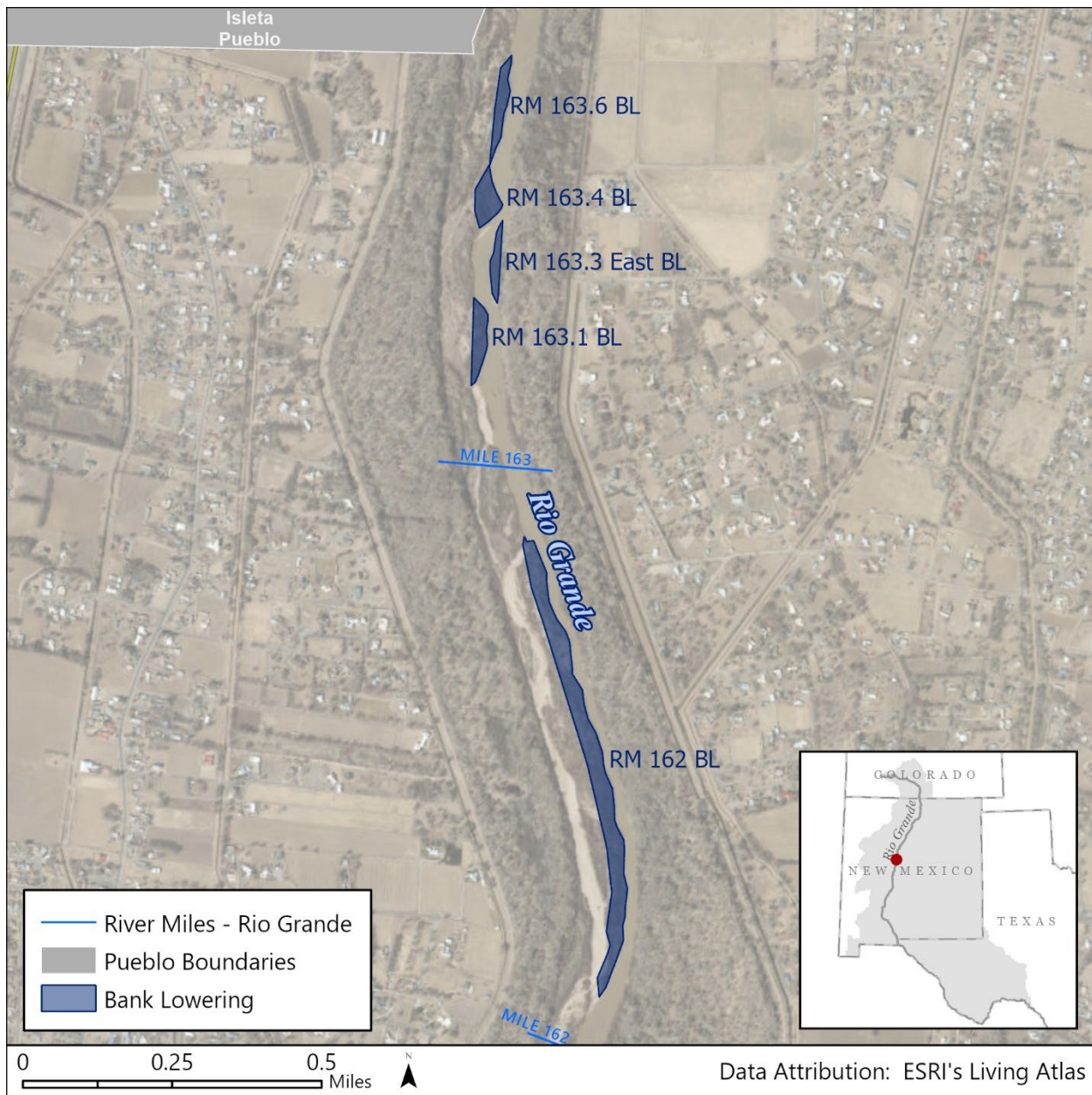
Figure 10: Plan view of bank lowering (BL) berm design for RM 163 maintenance project.
