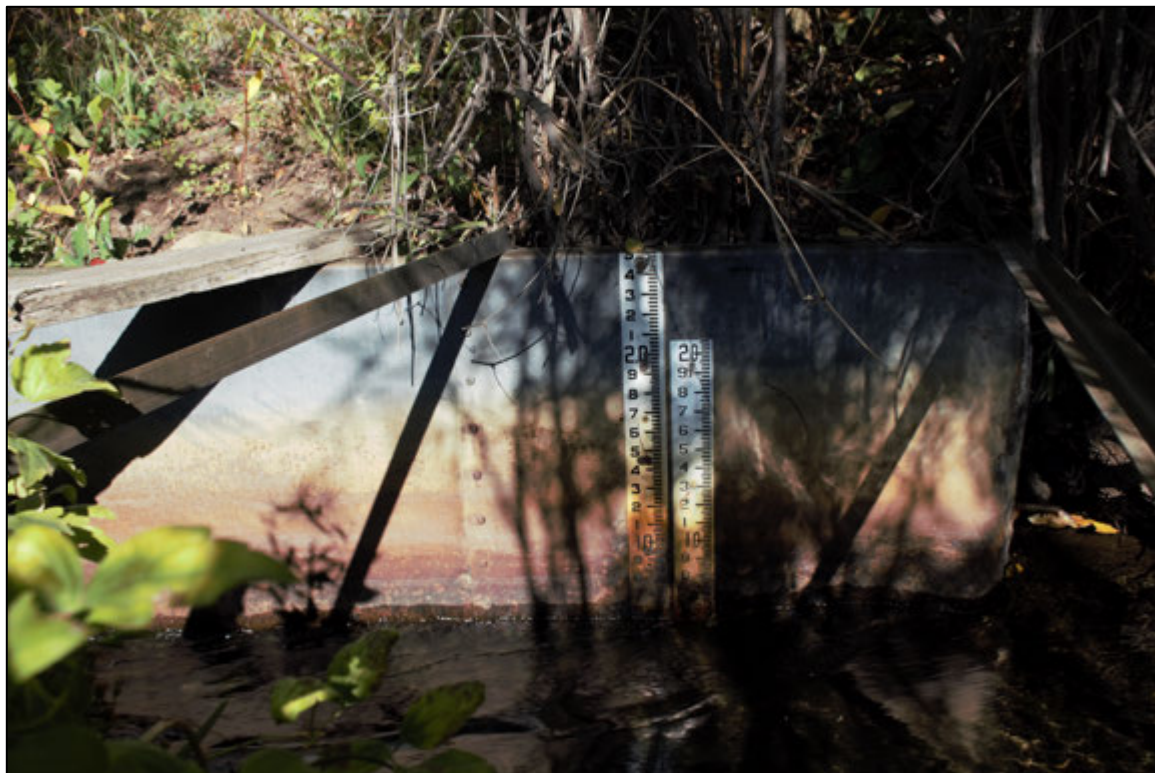
Figure 27. Gauge rulers on the north interior face of the Parshall Flume in Feature 3.
