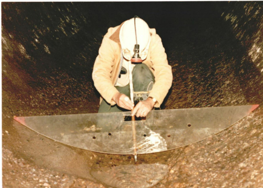
Photograph No. 35 - San Juan-Chama Project -- Blanco Tunnel - Photograph of Charles Fisher measuring the tunnel invert erosion using template and measuring device.
