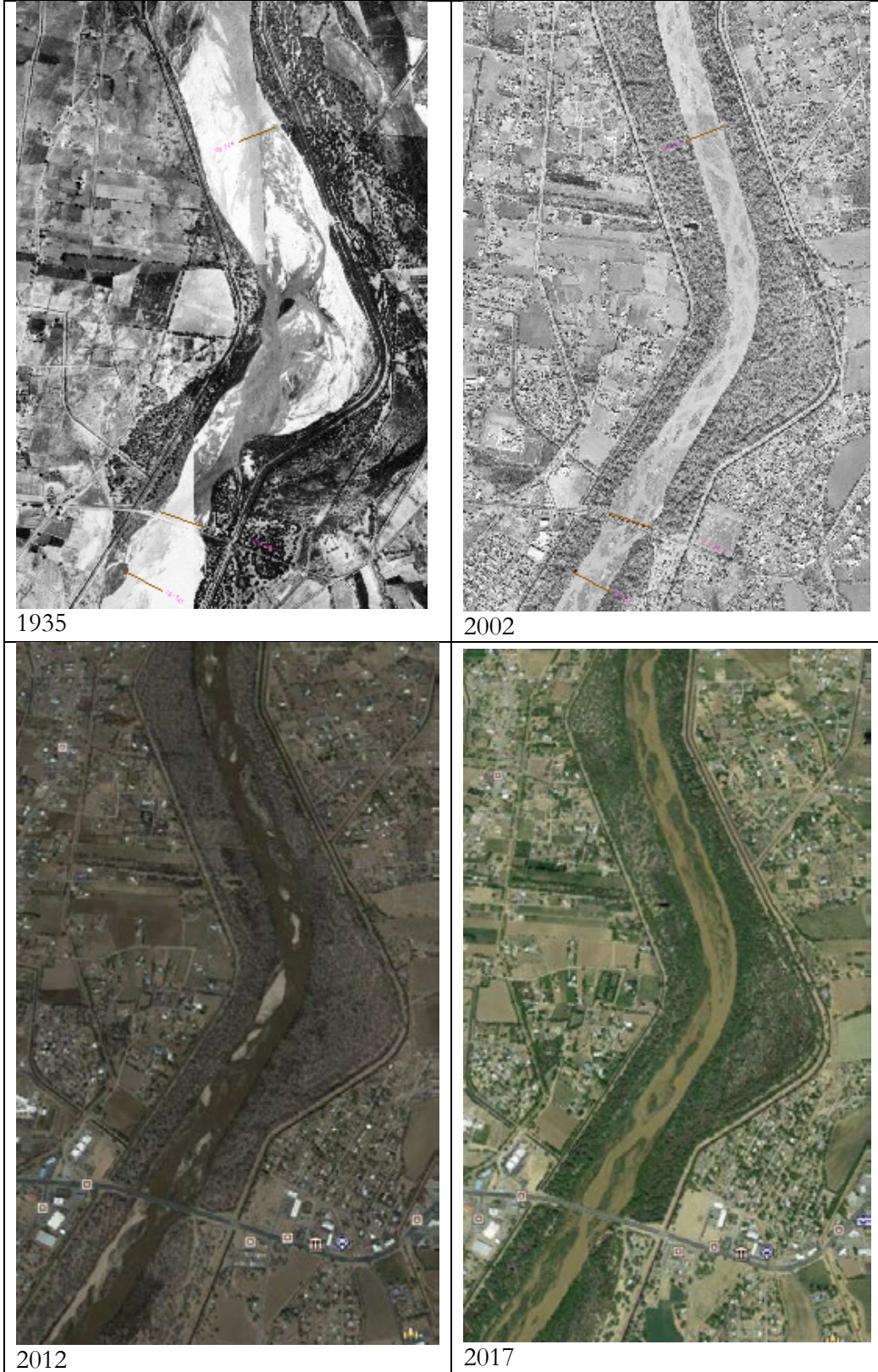
Figure 6: Planform channel changes for Los Lunas NM-6 bridge area for 1935, 1962, 2012, and 2017
