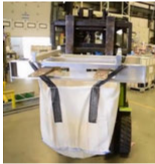
Bag Removed by Forklift
