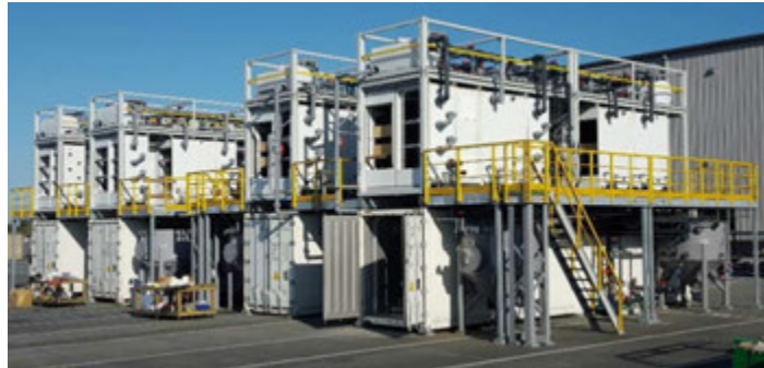
S100 + S125 SaltMaker Plants Capacity Increased by adding a S125 plant block 100 m 3 /day + 125 m 3 /day = 225 m 3 /day freshwater removed capacity
