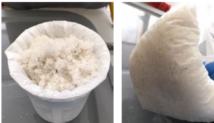
Figure 9: Field Paint Filter Screening Test for Solids - Passed after 48 hours of Dewatering
