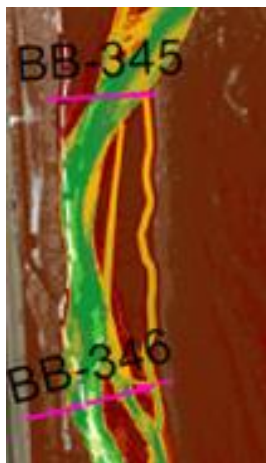
Figure 36: Topography map showing example design of limited side channels (orange) on the RM 199 point bar (red)
