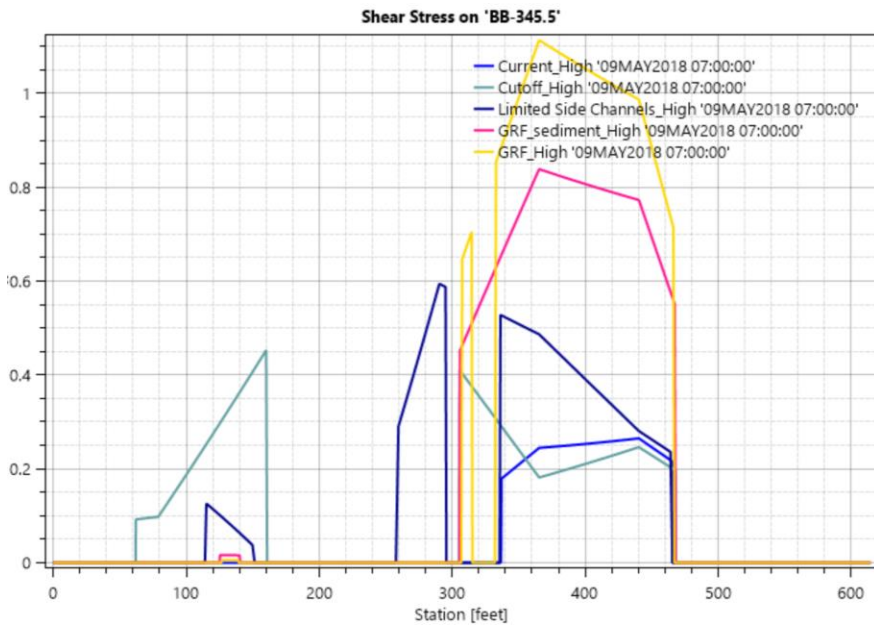
Figure 56: a) Cross section of terrain for all four models on BB- 345.5 and, b) Shear Stress at BB-345.5
