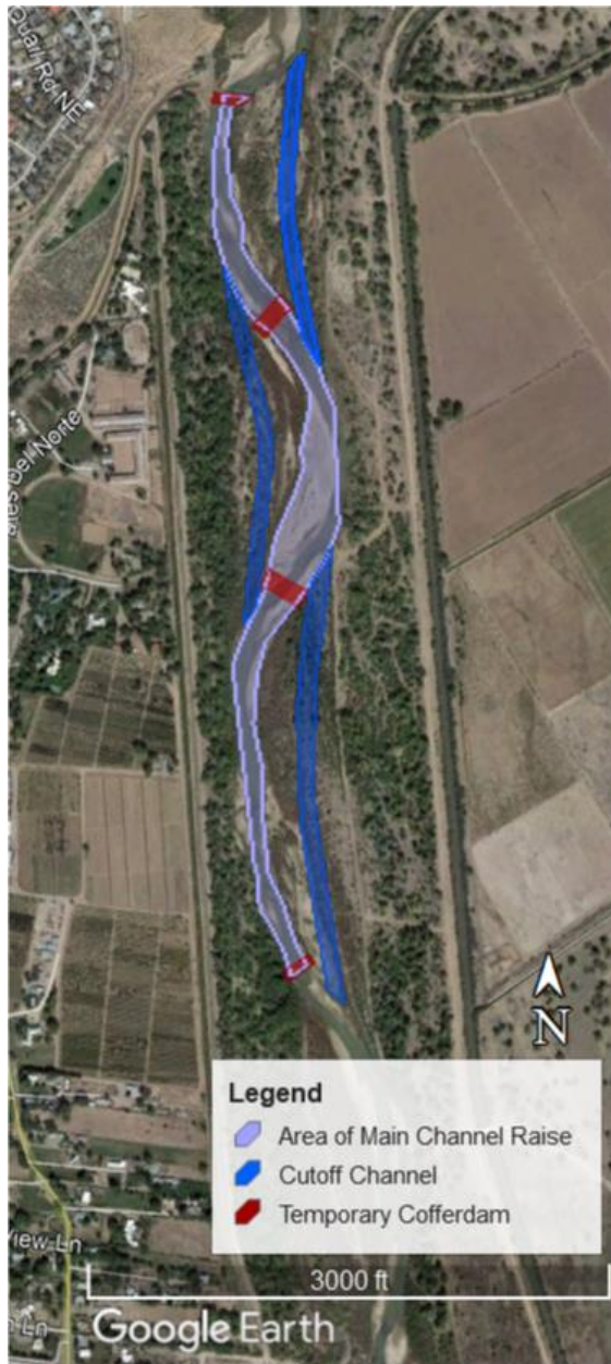
Figure 33: Cutoff channel alternative components, zooming in on the three upper bends to better demonstrate details
