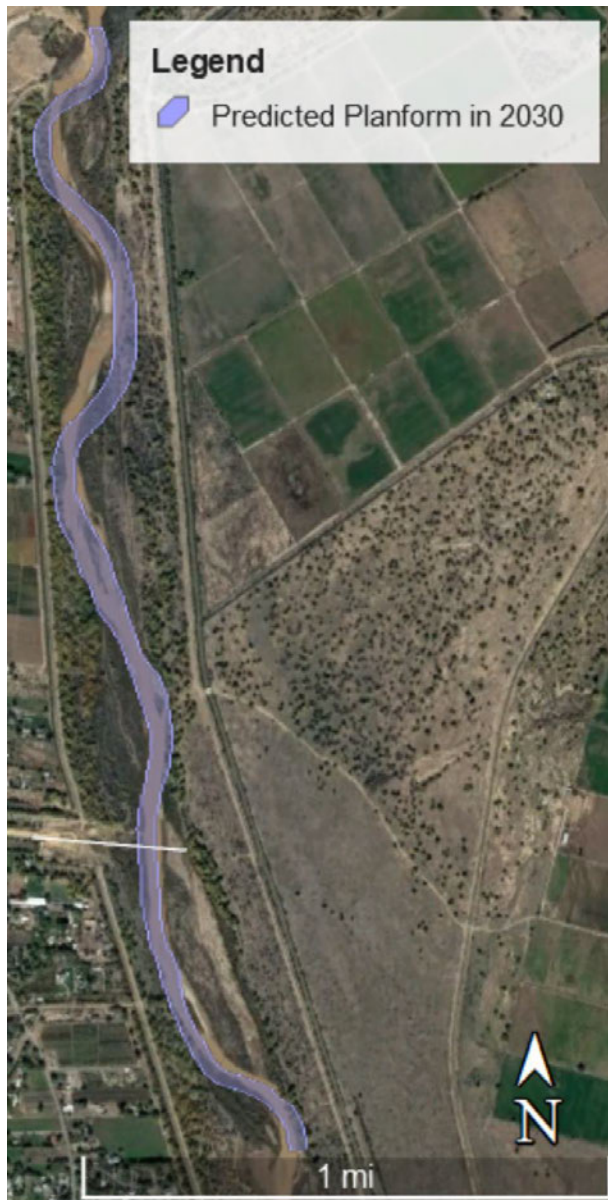
Figure 37: Predicted planform for year 2030 based on erosion rate and direction between 2013 and 2020
