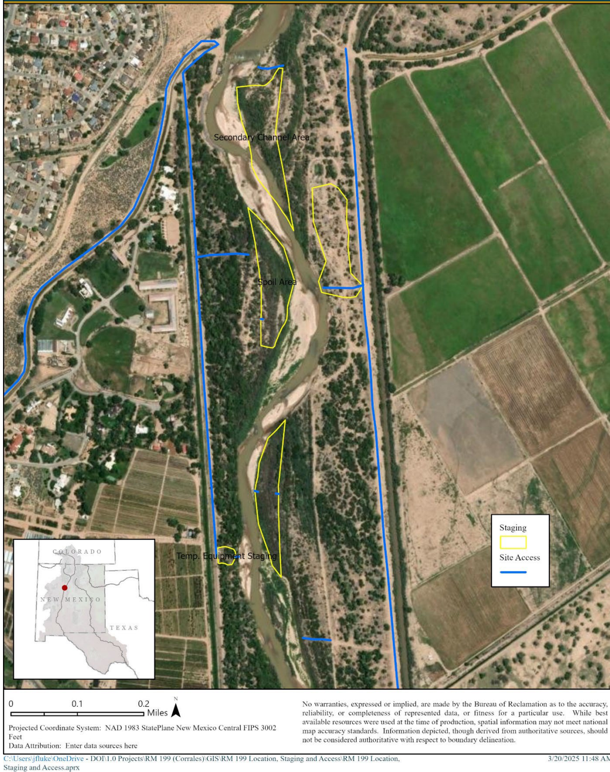
Figure 7: Plan view of project area showing the planned access routes and staging areas.
