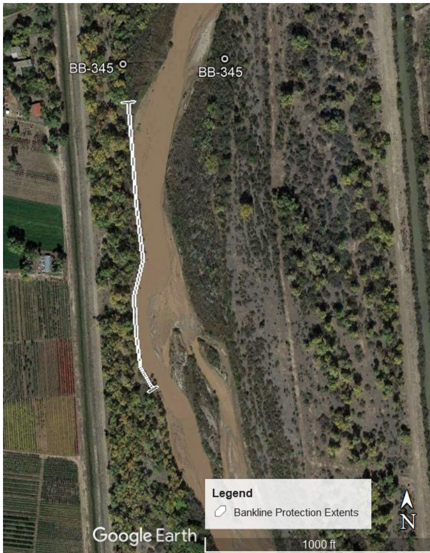
Figure 25: Extents of proposed bankline protection at the RM 199 bend, not including the structural keys and tie backs
