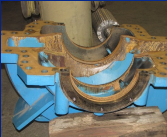
Damaged and Repaired Pump Coatings, Durango Pumping Plant, 2011
