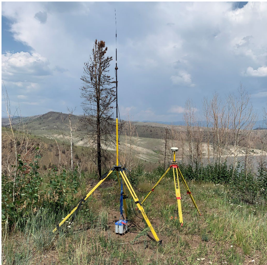
Figure A-2.—The RTK-GPS base station setup used during the survey of Willow Creek Reservoir in Colorado.
