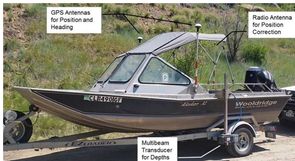
Figure A-1.—Wooldridge boat with real-time kinetic Global Positioning System (RTK-GPS) and multibeam depth sounder system (Odom MB-1 sonar transducer shown).
