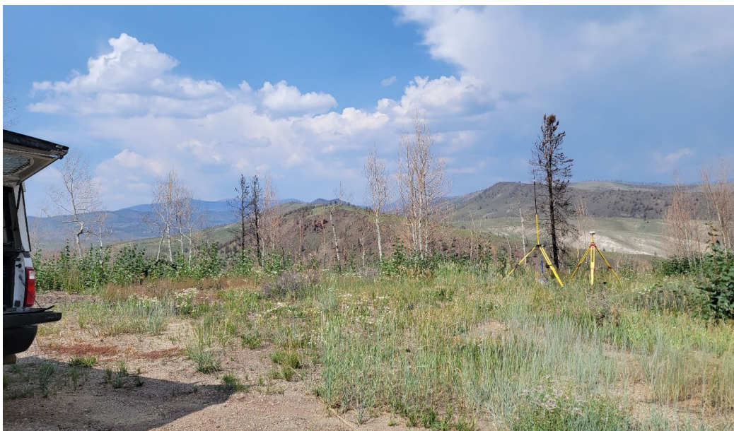
Figure 9.—GPS base station set up over the new benchmark (note burned tree in the background).
