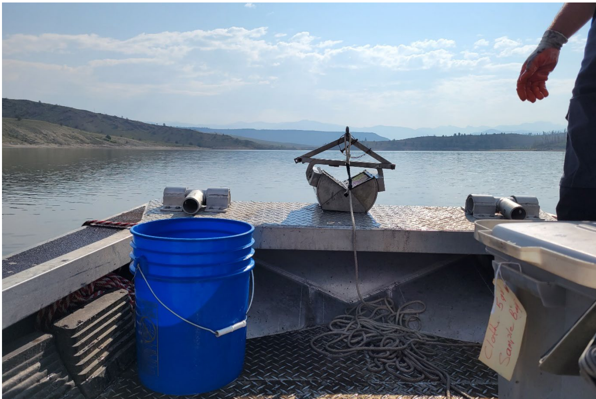
Figure 11.—Photograph of the PONAR sampler (on the bow of the boat) used to collect the reservoir bottom sediment samples.
