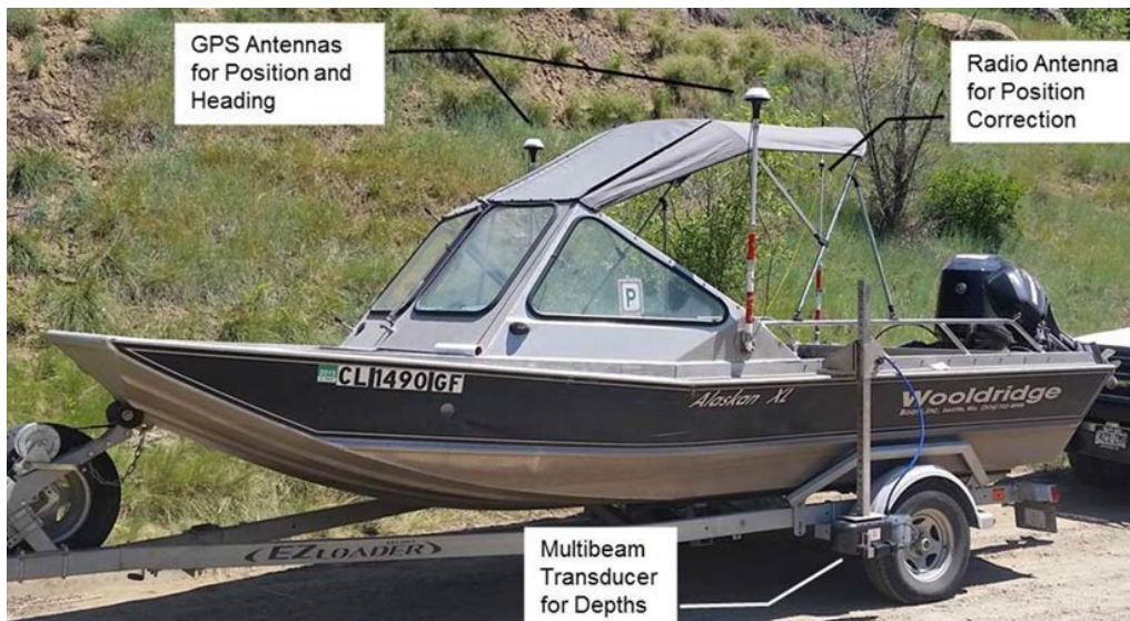
Figure 17. Wooldridge boat with RTK-GPS and multibeam depth sounder system.
