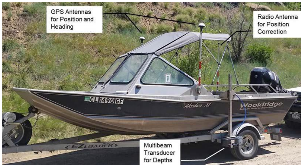
Figure 16. Wooldridge boat with RTK-GPS and multibeam depth sounder system.
