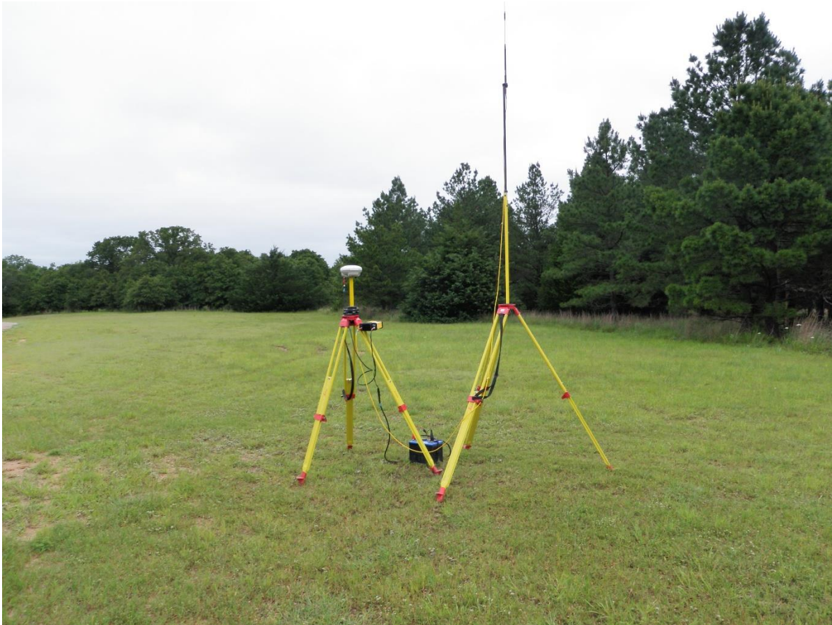
Figure 17. The RTK-GPS base station set-up used during the survey.
