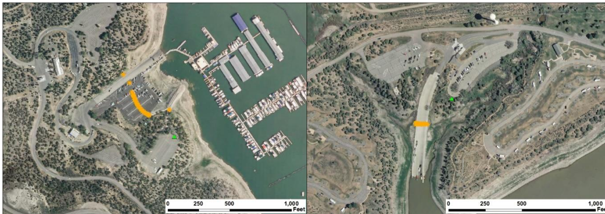
Figure 9. Location of GPS base stations and WSE points collected near marinas. Green triangles are base station locations and orange asterisks are WSE points.
