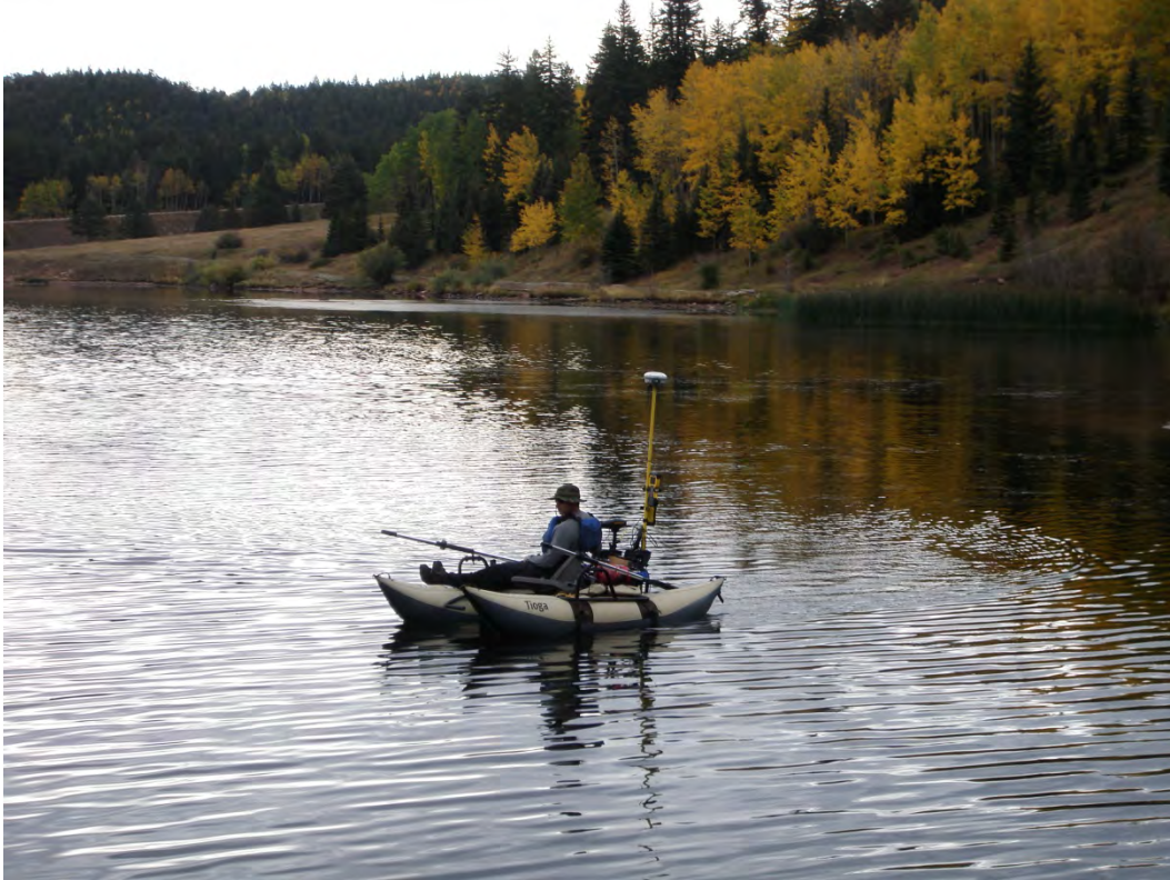
Figure 11 - Vessel used to collect depth data along the shoreline of Lake Isabel.
