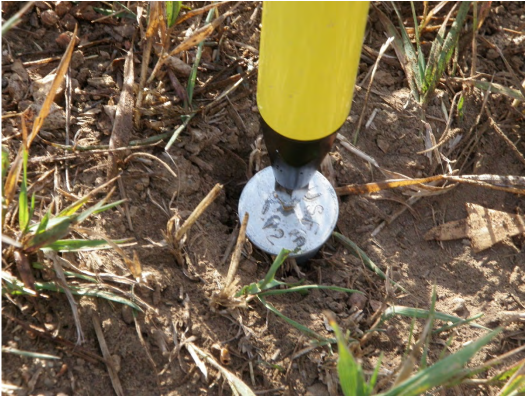
Figure 4 - USFS-1 09-12: Aluminum cap on rebar.
