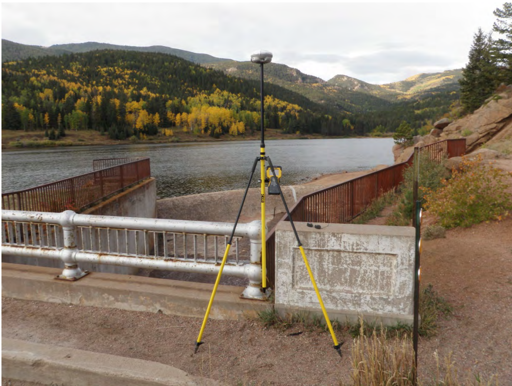
Figure 9 - Center of northeast bolt of spillway channel rail.
