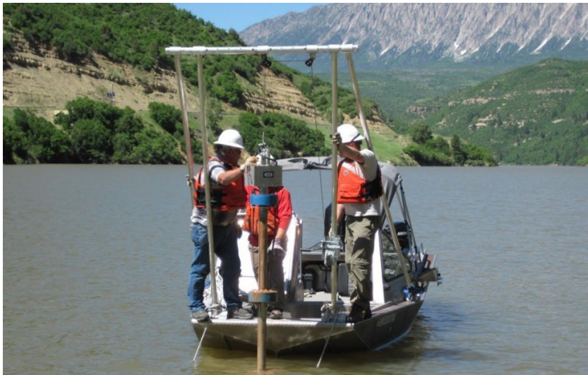
Figure 6. Photograph of sediment sampling from Paonia Reservoir near Paonia, Colorado using the VibeCore-4D vibrating core (vibracore) sampler (manufactured by Specialty Devices Incorporated).
