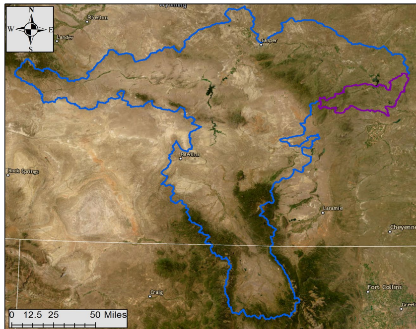
Figure 3.—The watershed above Guernsey Reservoir has a total drainage area of 15,853 mi 2 (blue outline) and a sediment-contributing drainage area of 675 mi 2 (purple outline). Dams upstream of Guernsey include Glendo, Alcova, Pathfinder, and Seminoe and trap sediment from most of the basin.
