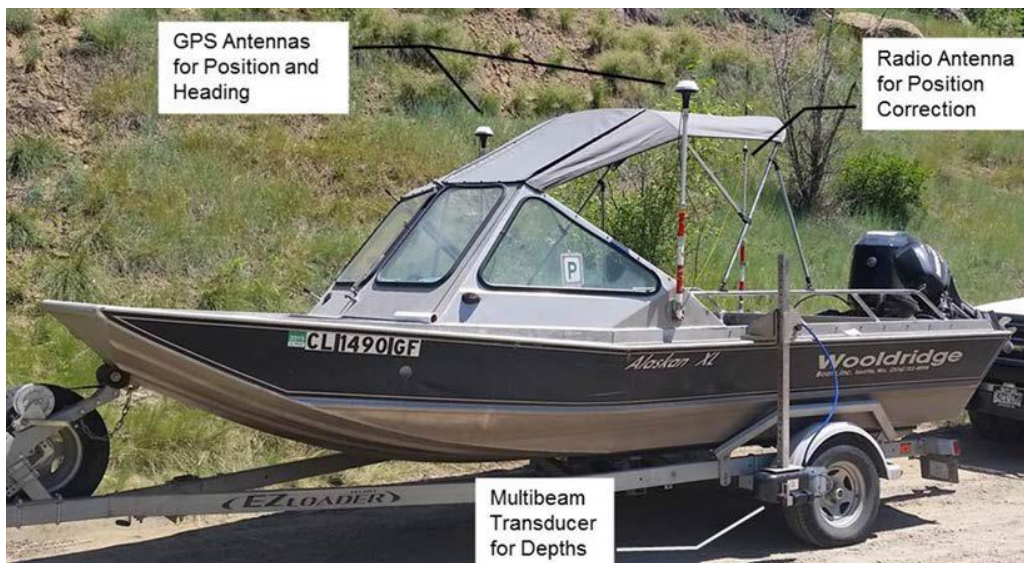
Figure 19. Wooldridge boat with RTK-GPS and multibeam depth sounder system.
