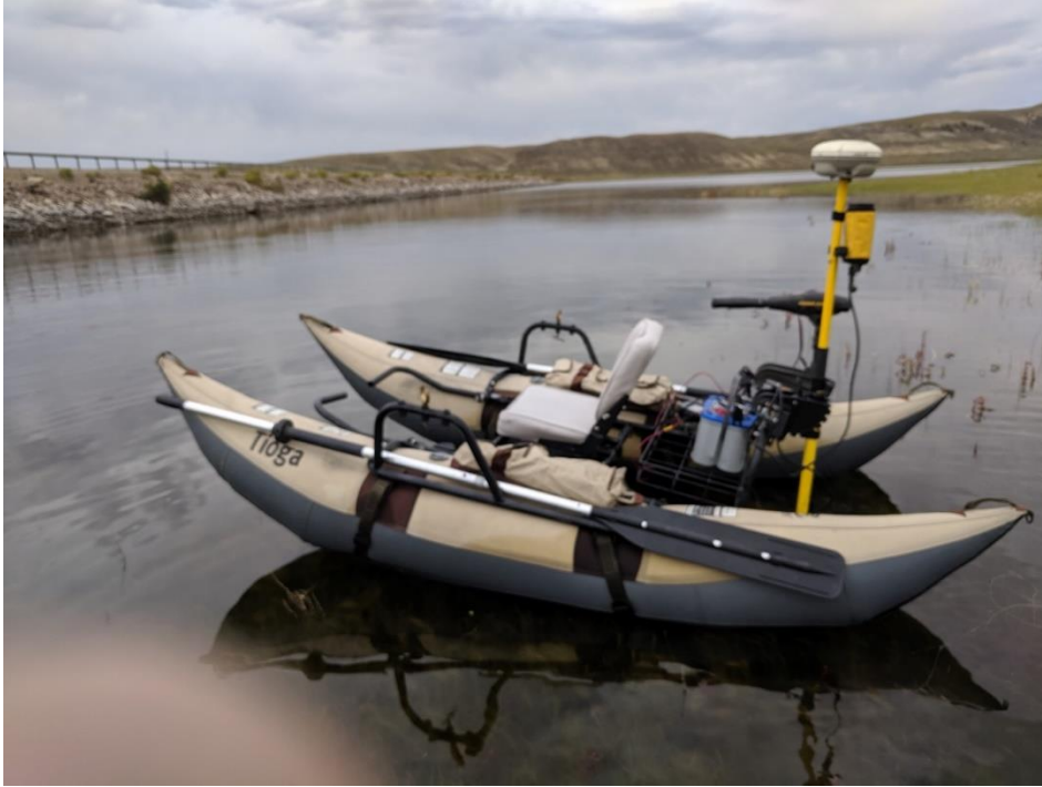
Figure 21. Cataraft survey boat on the Fontenelle Creek arm of the reservoir with RTK-GPS and single beam depth sounder.
