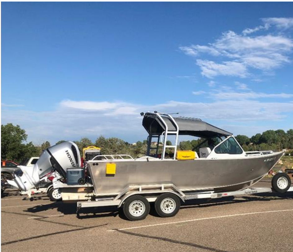
Figure 20. WCAO survey vessel used to measure depths using an ADCP instrument.
