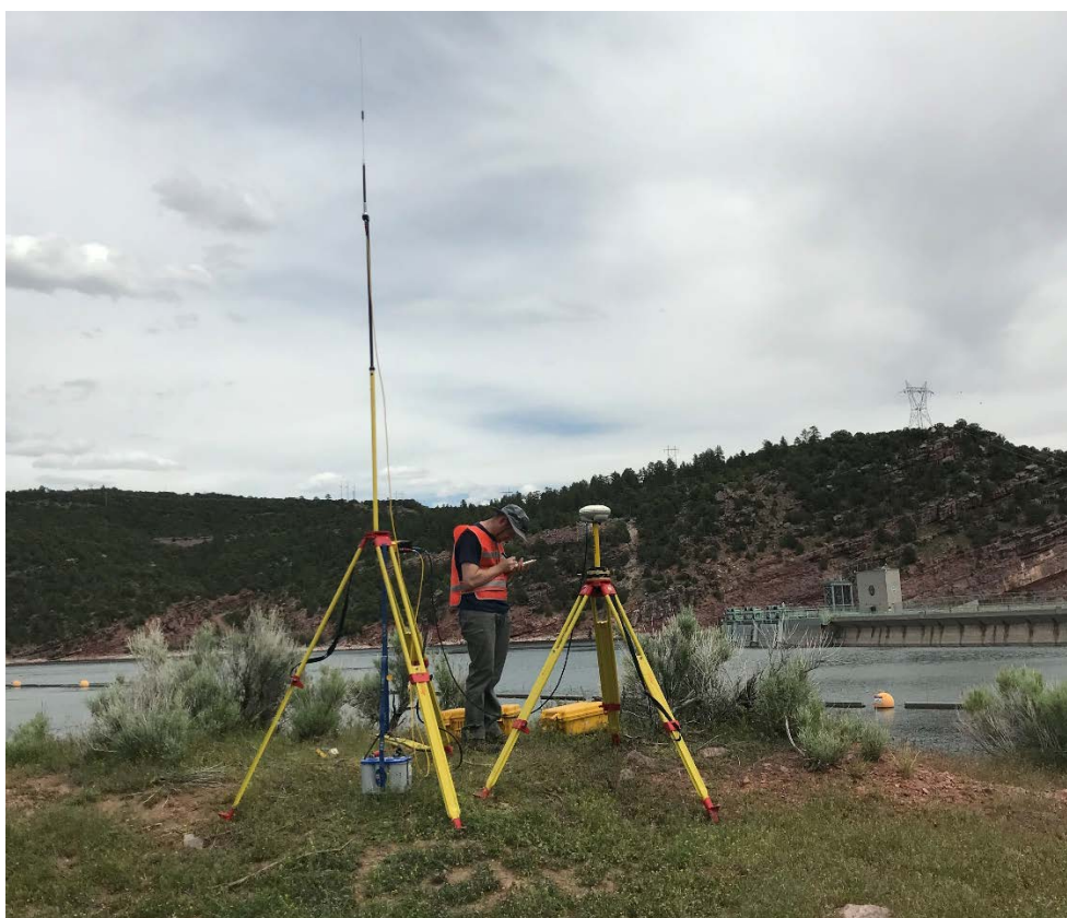
Figure 37. The RTK-GPS base station set-up used during the survey El Vado Reservoir in New Mexico is typical of the set up used for other reservoir surveys.
