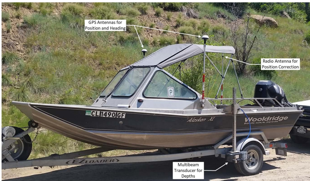
Figure 36. Wooldridge boat with RTK-GPS and multibeam depth sounder system.
