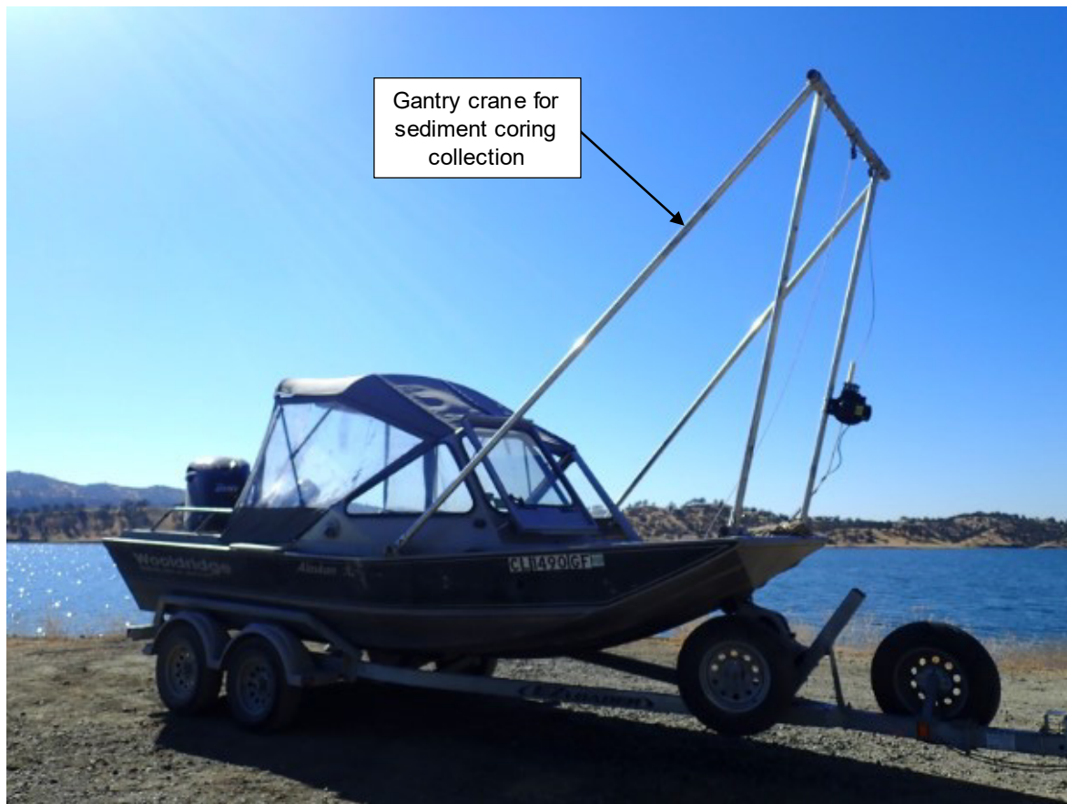
Figure A-2.—Survey vessel equipped with gantry crane for sediment coring.
