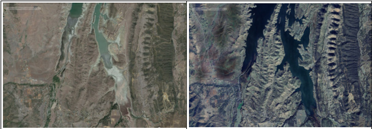
Figure 2.—Deltas from the Little Stony and Indian Creek inflow. The left image shows a low reservoir water surface elevation (2021) while the right image shows a high reservoir water surface elevation (2023).
