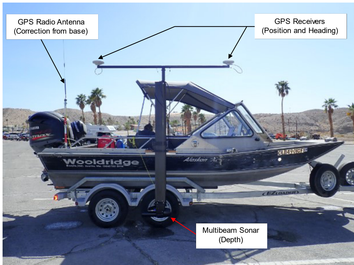
Figure A-1.—Survey vessel and multibeam system used for bathymetry collection.
