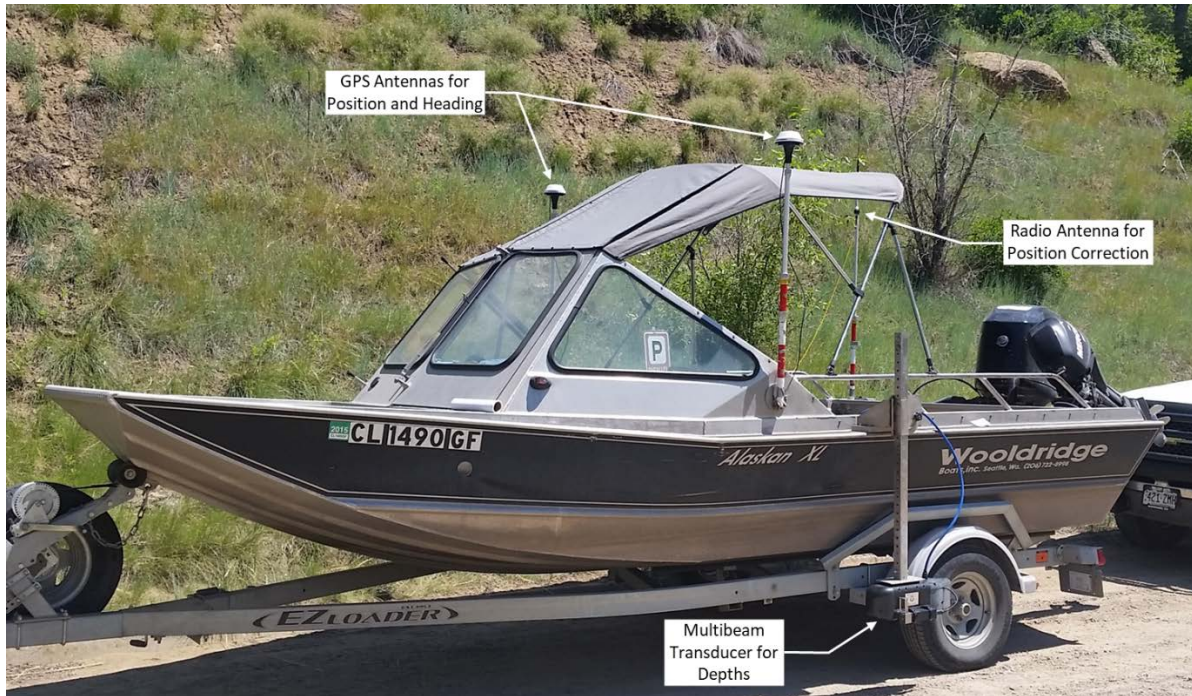
Figure 22. Wooldridge boat with RTK-GPS and multibeam depth sounder system.
