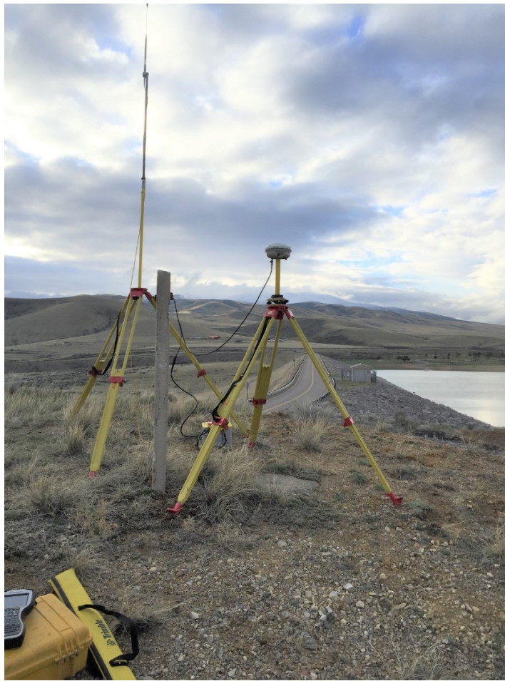
Figure 8. GPS base used during 2016 Clark Canyon bathymetric survey. Survey monument, brass cap set in concrete, shown directly under the GPS receiver (right) tripod
