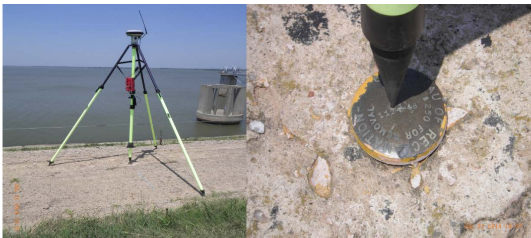
Figure 8. Survey marker designated "112+46" on Cheney Dam crest used to verify 2015 GPS measurements. Photos courtesy of Orosco (2014).
