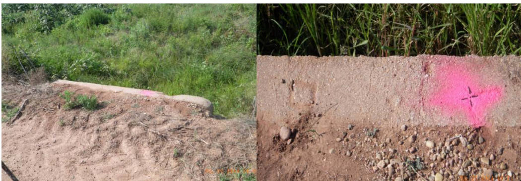
Figure 5. CR-37 "X" chiseled in concrete near east end of Range 5 used to verify 2015 GPS measurements. Photos courtesy of Orosco (2014).
