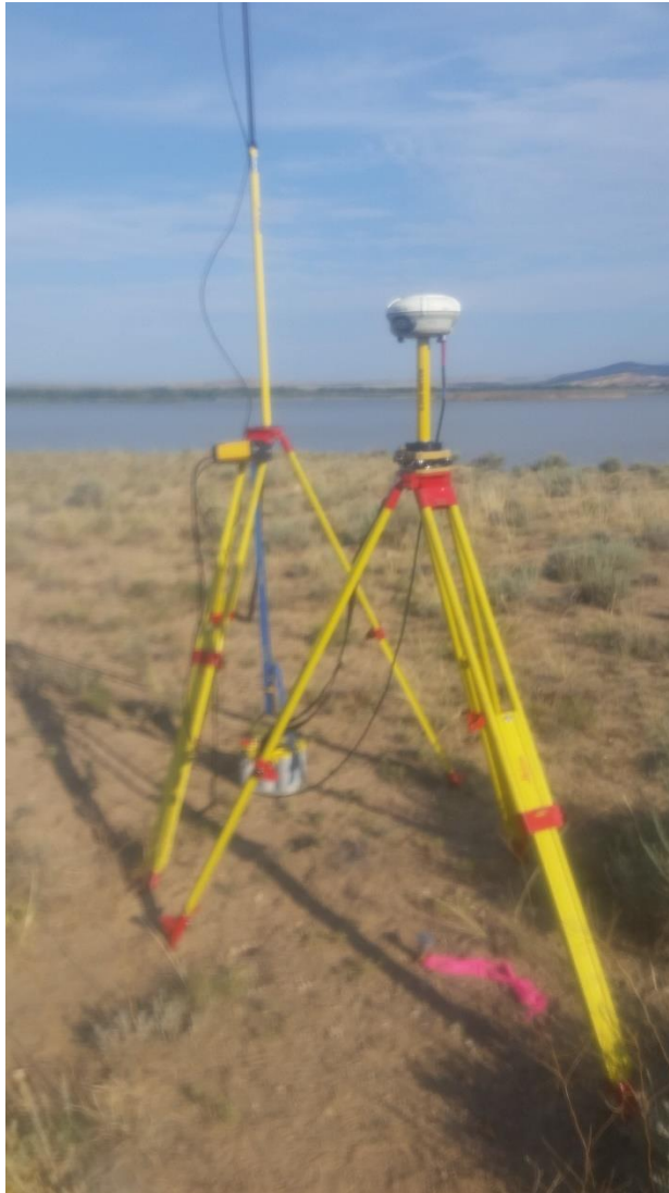
Figure A-3. The RTK-GPS base station set-up used during the survey of Bighorn Reservoir (photo by Kent Collins).
