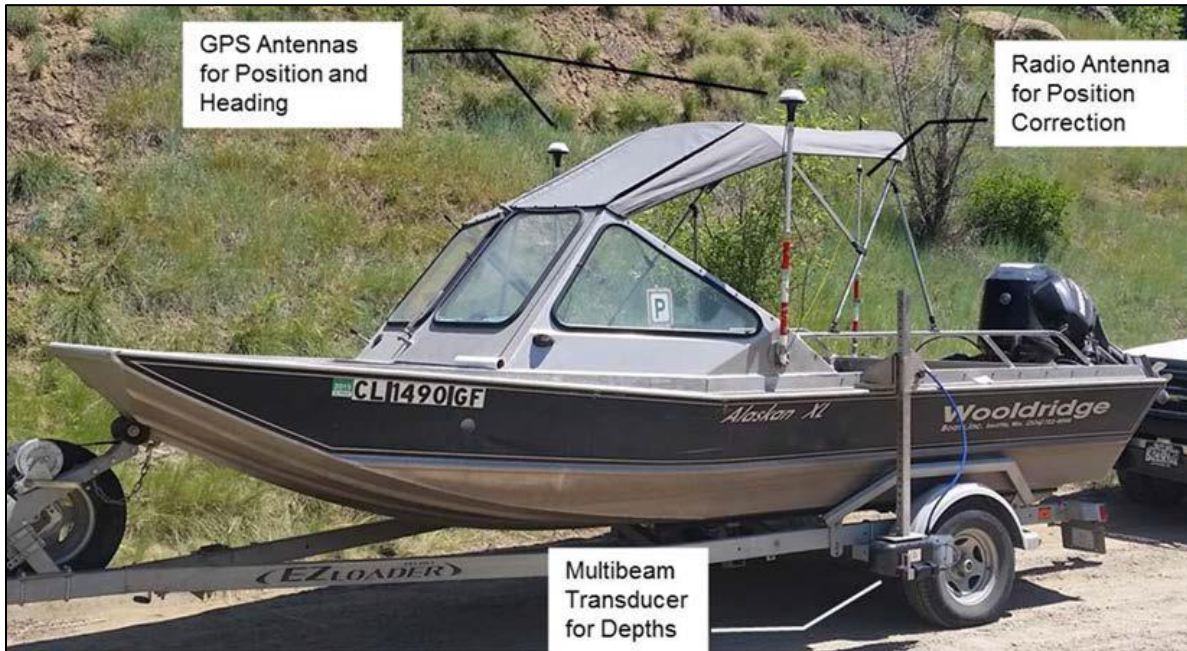
Figure A-1. Wooldridge boat with RTK-GPS and multibeam depth sounder system (Photo by Kent Collins).
