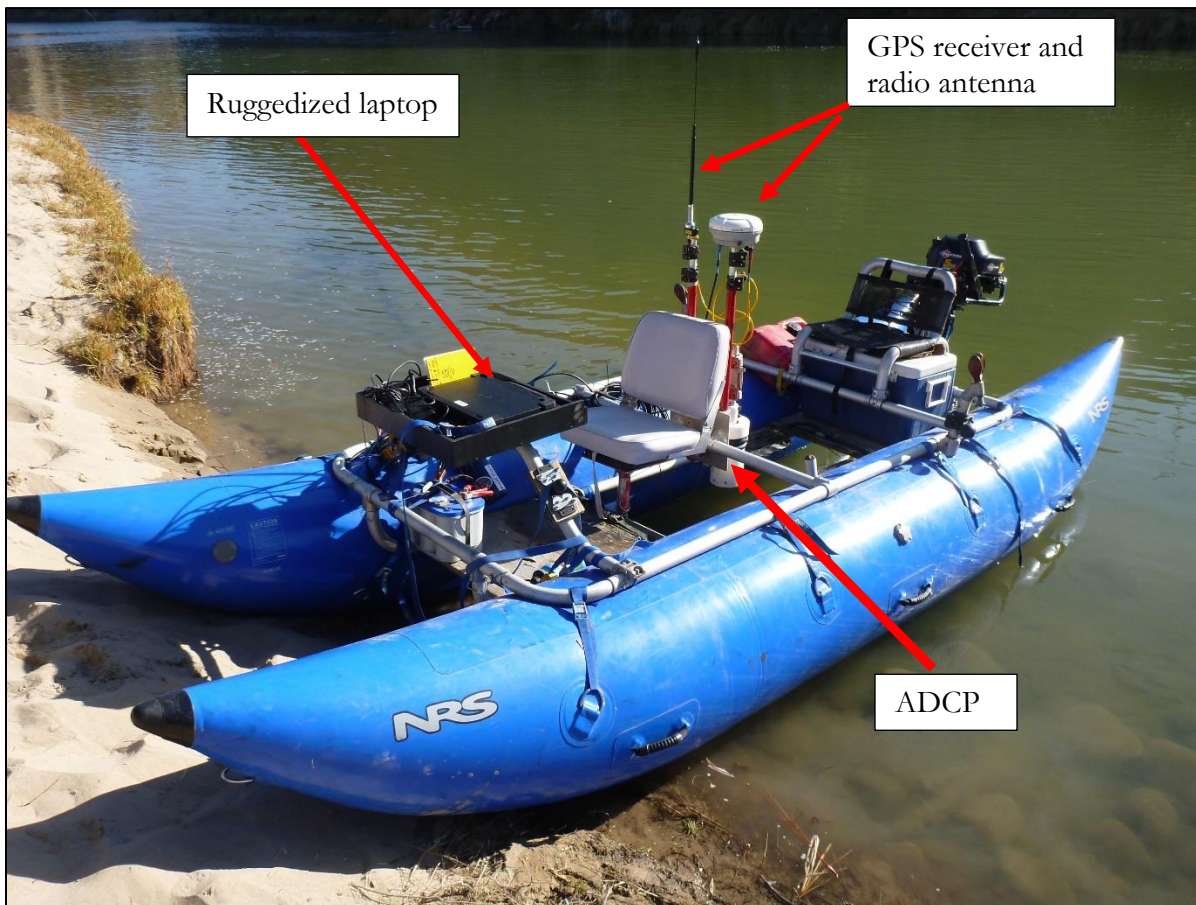
Figure A-2. Photo of a cataraft rigged for bathymetric surveying (Photo by Reece Carpenter).
