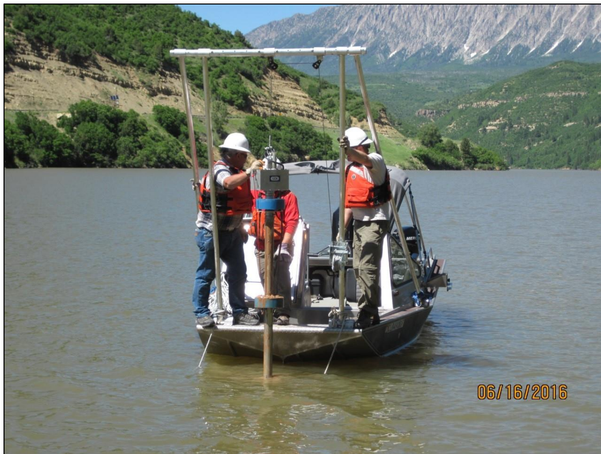
Figure 9. VibeCore sampling configuration mounted to the bow of an 18-foot aluminum boat (photo by Kent Collins).
