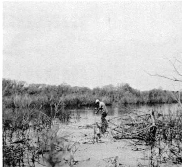
Figure 11. Sediment sample being taken by pounding a plastic tube into the sediment deposits with a rubber mallet. Photo P258-D-57702
