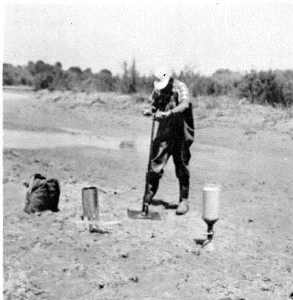
Figure 12. Taking a sediment sample with field density apparatus. Photo P258-D-57697
