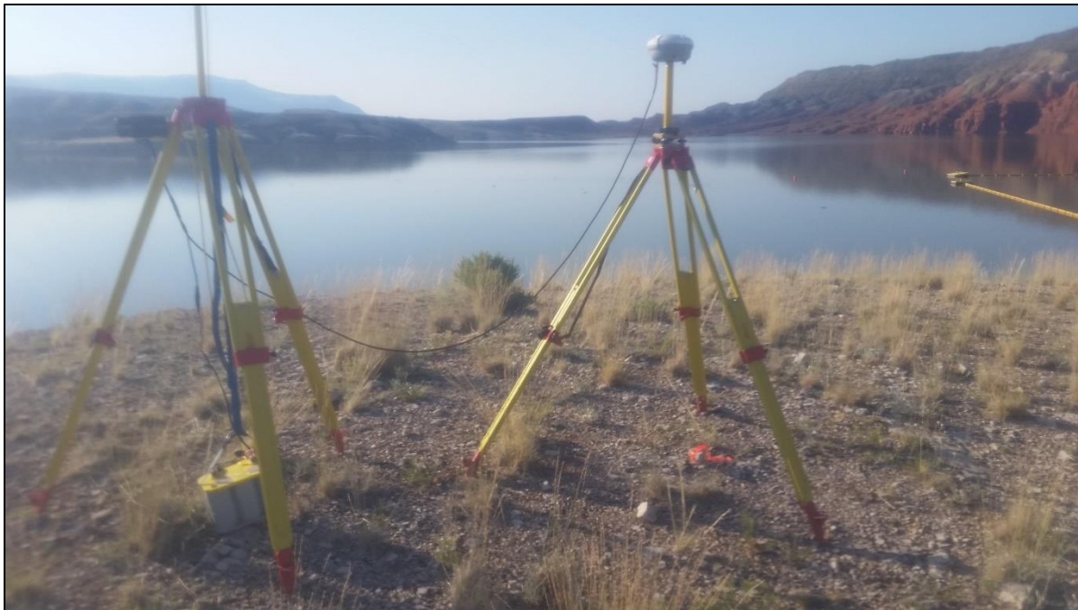
Figure A-2. The RTK-GPS base station set-up used during the survey of Bighorn Reservoir in Montana is typical of the set up used for other reservoir surveys.
