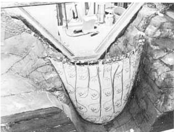
Figure 20.—Strain gages on upstream face—Morrow Point model.
