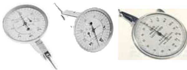
Figure 16.—Dial gages used for measuring model deflections.
