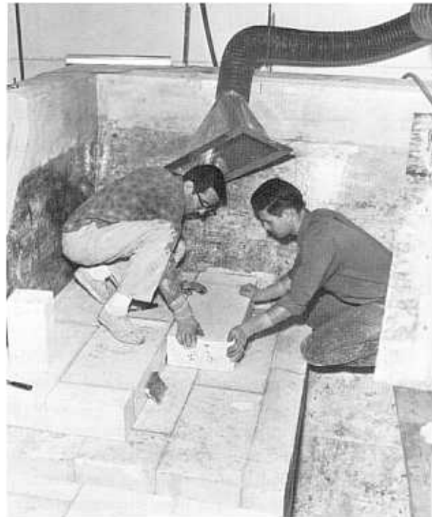
Figure 6.—Model construction by the block method—Morrow Point model.
