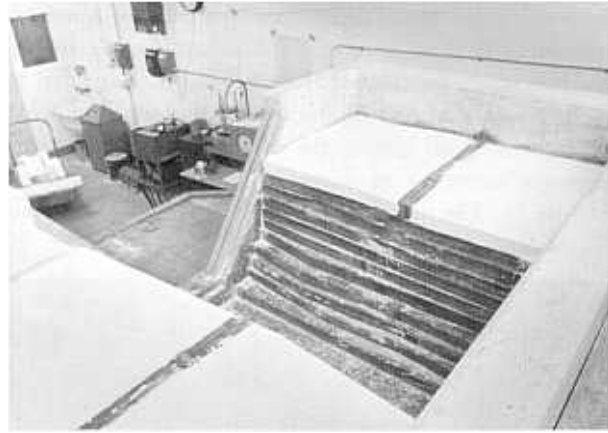
Figure 5.—Model construction by the layer method—Glen Canyon model.
