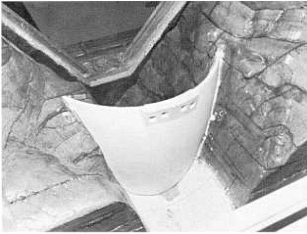
Figure 10. —Model of Morrow Point Dam in place.
